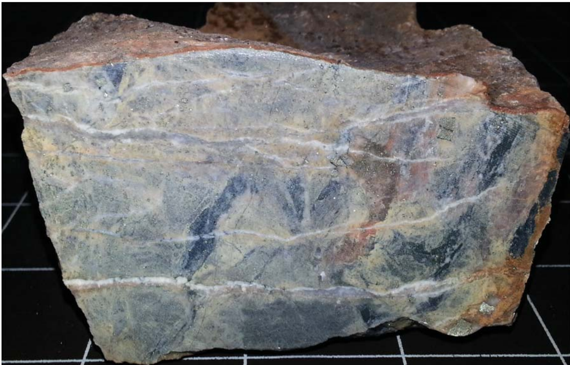
Plate 1: Trachybasalt grab sample from Rollo Twp property. Note pervasive alteration of basaltic groundmass and intense carbonate veining. White squares = 3 x 3 cm.
