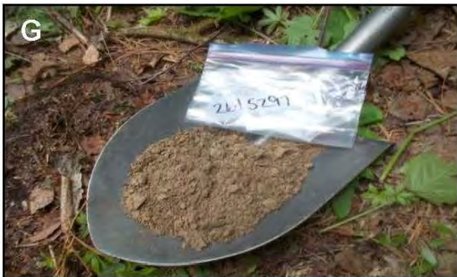
Figure 6: Field photos from the Midlothian Property showing (A) typical soil-sampling environment, (B) pit of brown silt, (C) mechanically aggregated pebbles and cobbles in a gravel pit, (D) rusty brown silt, (E) grey-brown silt, (F) pit of grey clayey silt, (G) grey clayey silt and (H) dark brown organic-rich soil.
