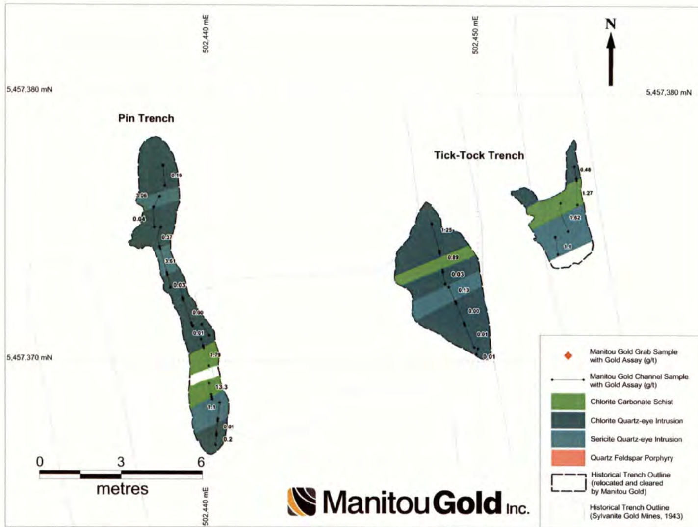
Figure 7.6: Pin and Tick-Tock trench geology maps showing locations of 2013 Channel samples. Assays are shown in g/t Au.
