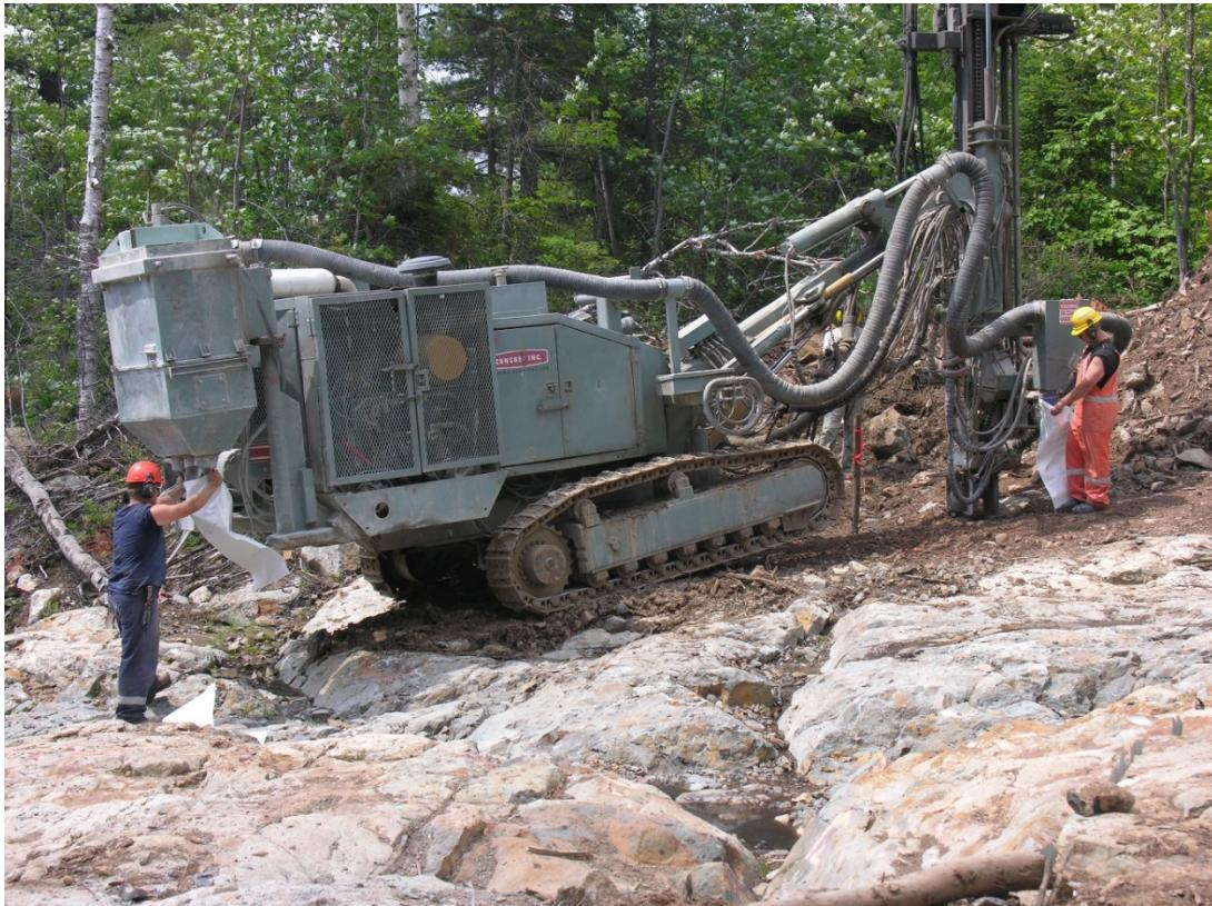
Gardiner Denver Model SCH 5000 collaring PD-14-03-N on the 007 Showing, July 22, 2014. BQTK diamond drill hole is marked by stake with red flagging tape.
