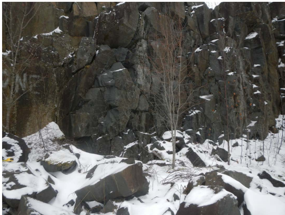
Photo 4: Quarry Site – Variable Jointing from Moderately to Widely Spaced
