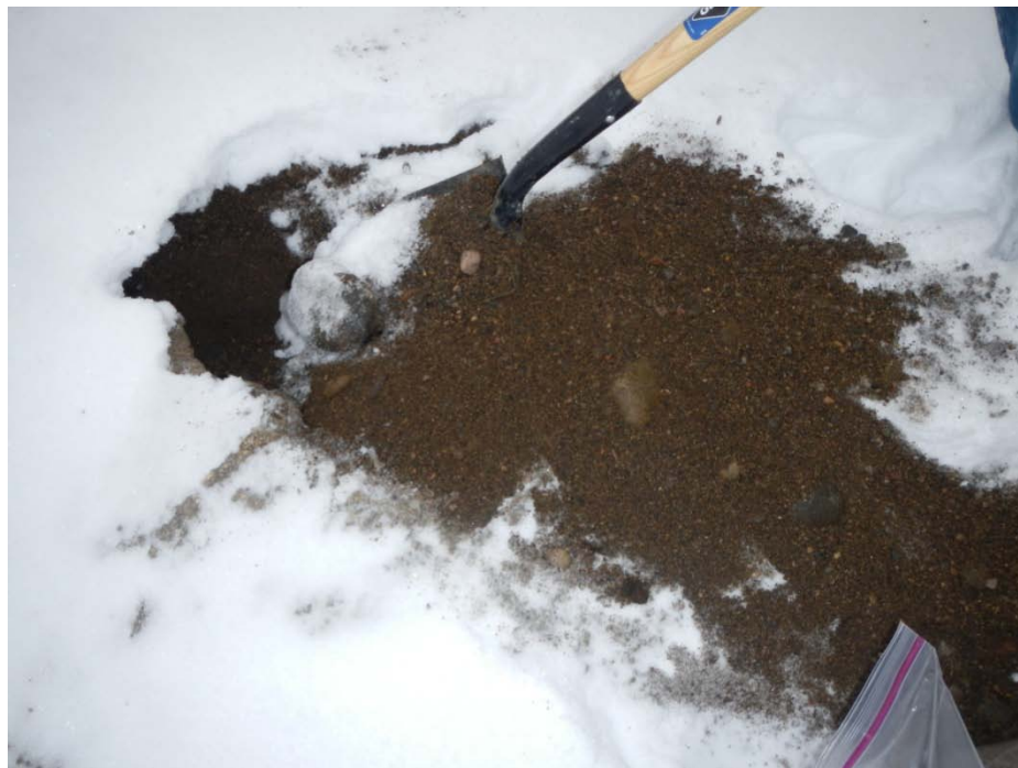
Photo 6: Borrow Pit Sample Containing Medium to Coarse Grained Sand and Fine Gravel with Trace Coarse Gravel
