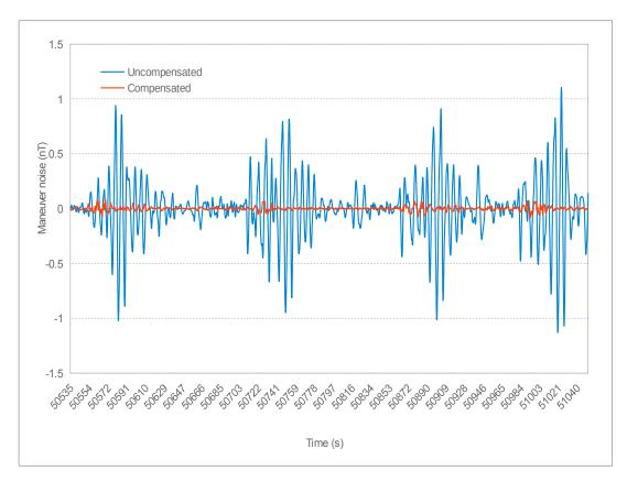
Figure 6: Mag 3 Tail Compensation calibration test
