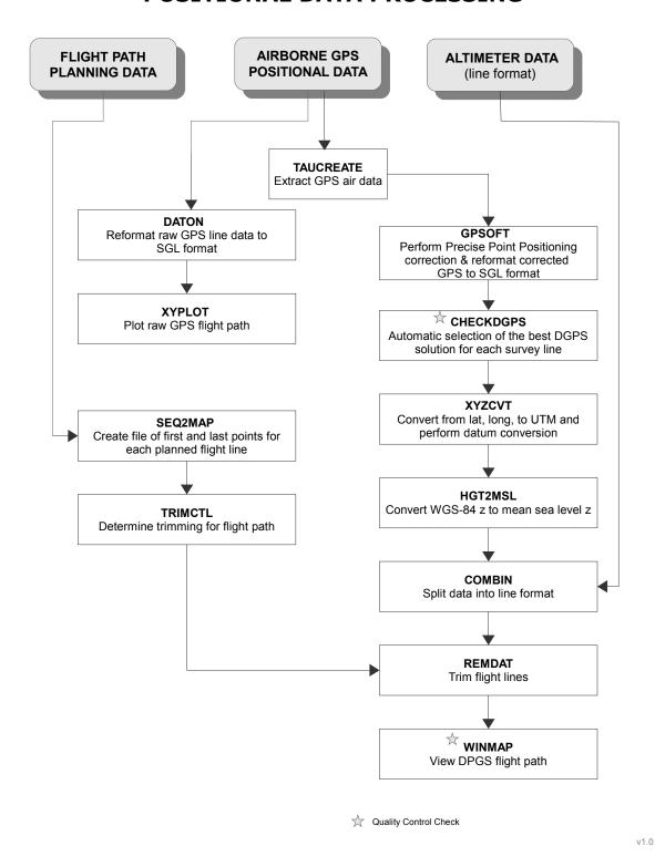
Figure 13: Positional data processing flowchart
