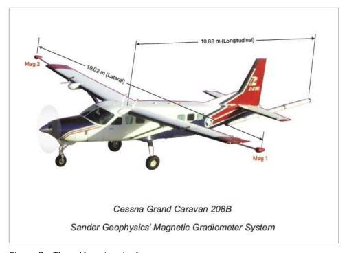
Figure 3: Three Magnetometer Array
