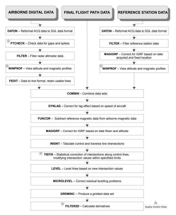
Figure 12: Magnetometer data processing flowchart
