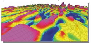
AIRGrav data: 3d image of the first vertical derivative of terrain corrected Bouguer gravity
