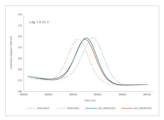
Figure 10: Mag3 Tail Magnetic Sensor Instrumentation lag test
