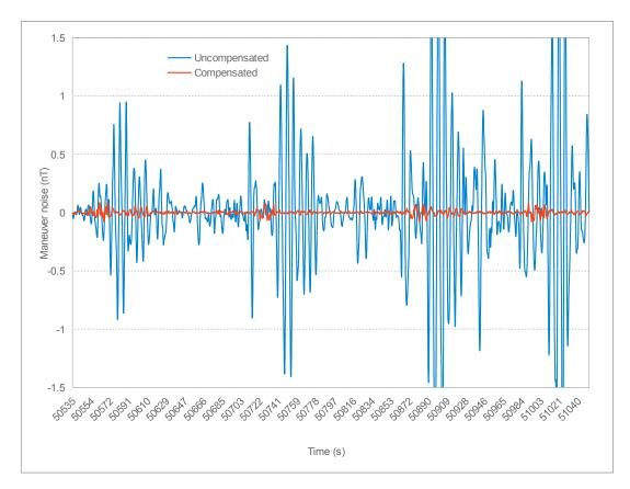
Figure 5: Mag2 Starboard Compensation calibration test
