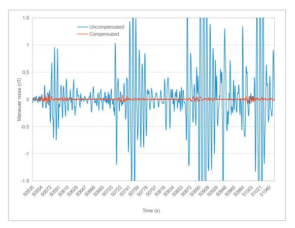
Figure 4: Mag1 Port Compensation calibration test
