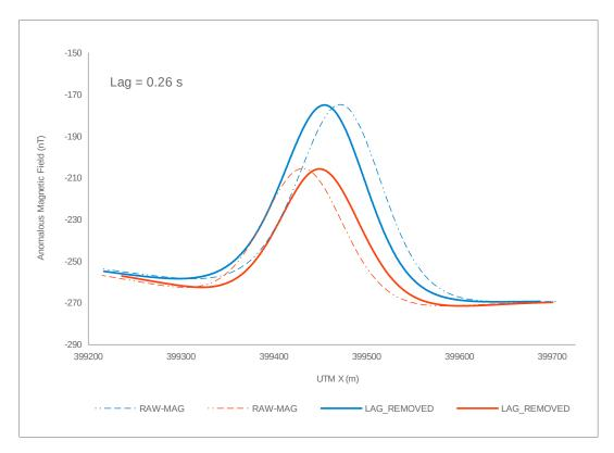
Figure 9: Mag2 Starboard Magnetic Sensor Instrumentation lag test
