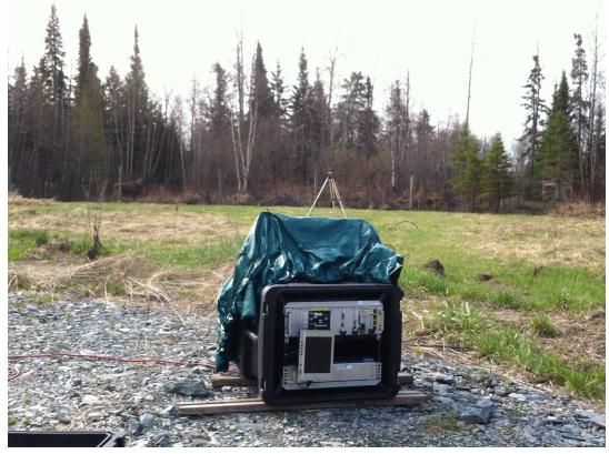
Picture 2: Reference station setup with GPS antenna in the background
