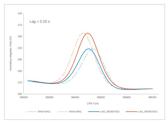
Figure 8: Mag1 Port Magnetic Sensor Instrumentation lag test
