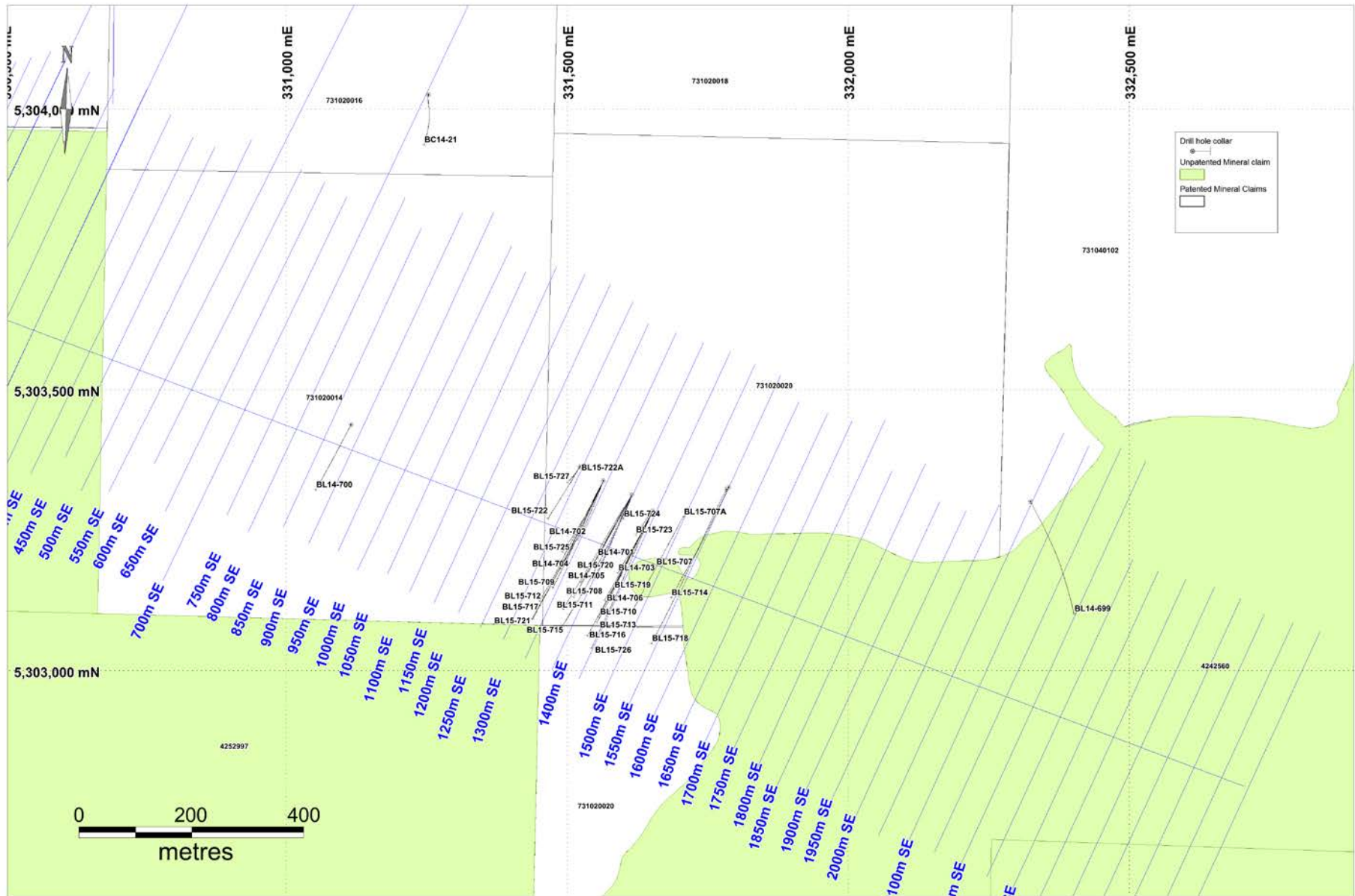
Figure 4 - Diamond Drill Hole Collar Locations and hole traces (see Appendix I for 1:4,000 map)
