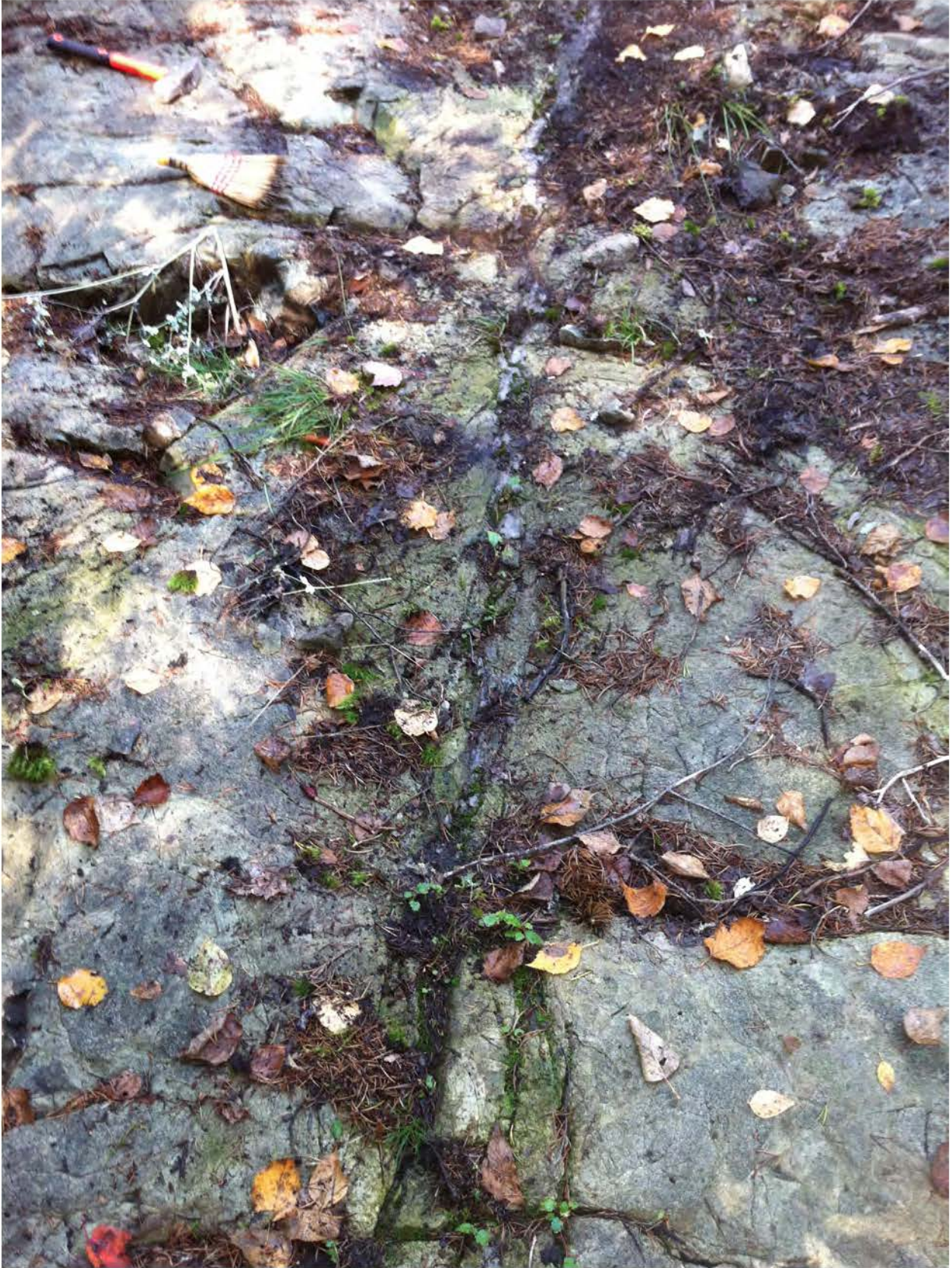
Photo 4: At WP 359 further east showing a quartz vein and adjacent brecciated rock.
