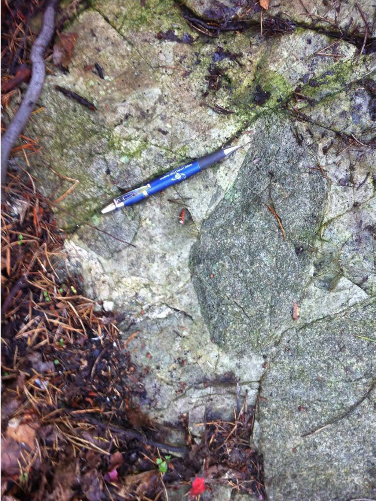
Photo 5: At WP359 showing gabbroic breccia fragments in a matrix of crushed gabbro.
