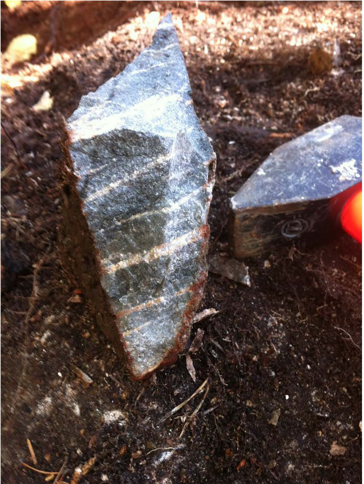
Photo 6: At WP 366 iron carbonate rich vein with later parallel quartz iron carbonate veins.
