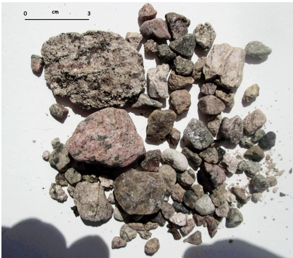
SEDIMENT SAMPLE AFTER MUD AND VEGETATIVE MATTER REMOVED
