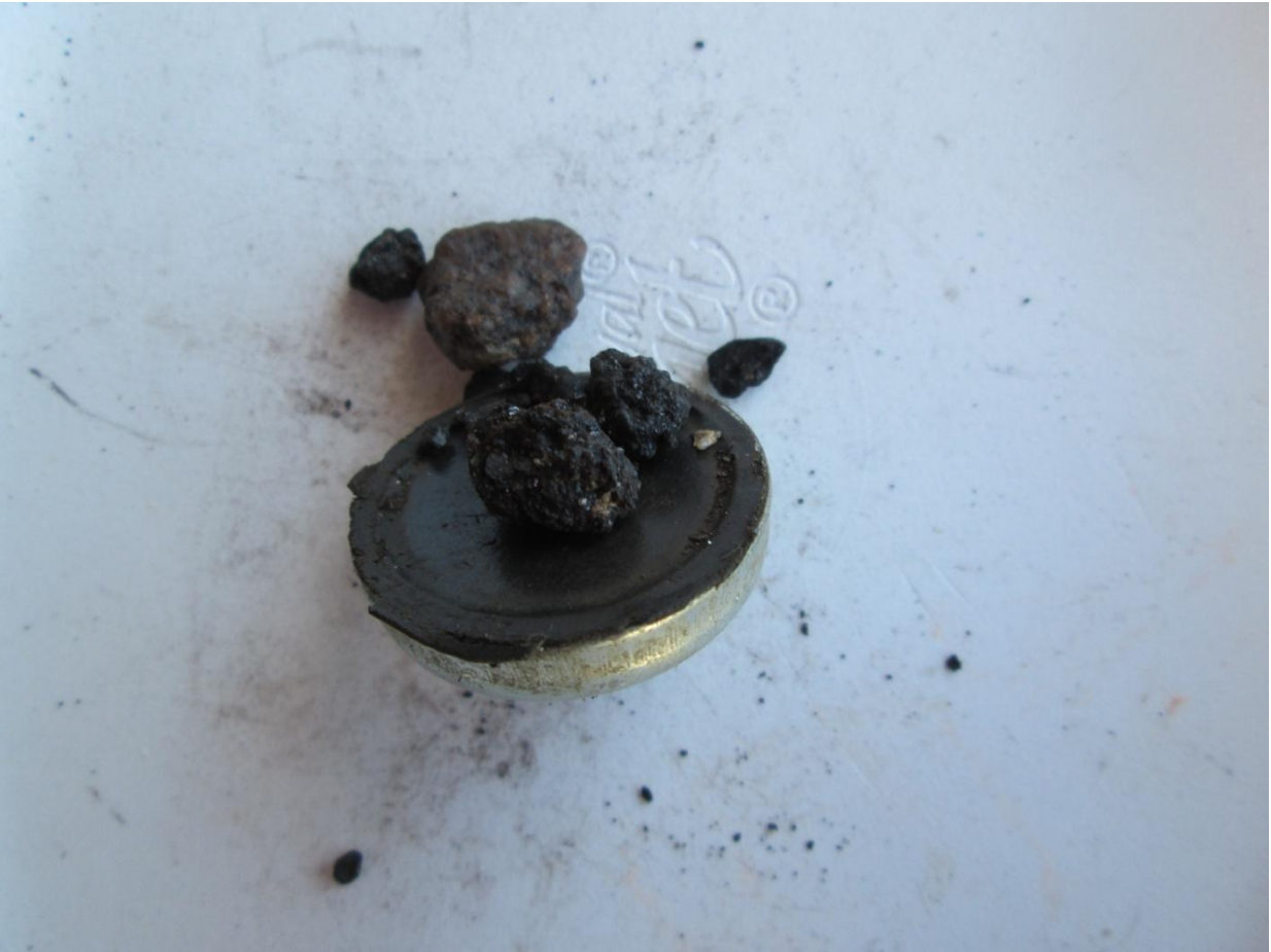
SAME GRAVEL ON MAGNET. (MAGNET IS 25 mm IN DIAMETER)
