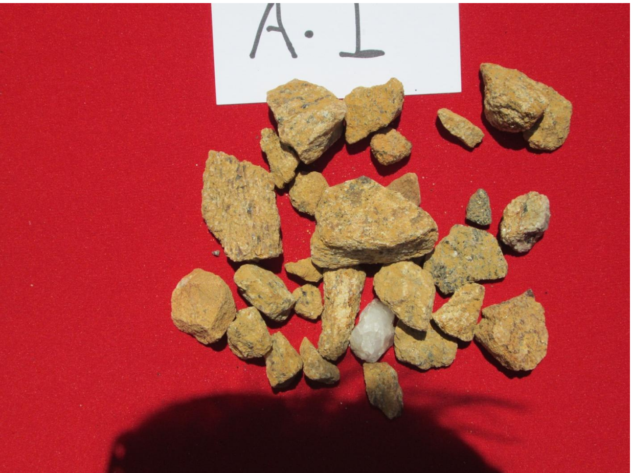
GRAVEL SELECTED FOR COLOR. CARD IS 8 cm WIDE THE TAN COLORED PEBBLES ARE PIECES OF CRUSTED PEGMATITE
