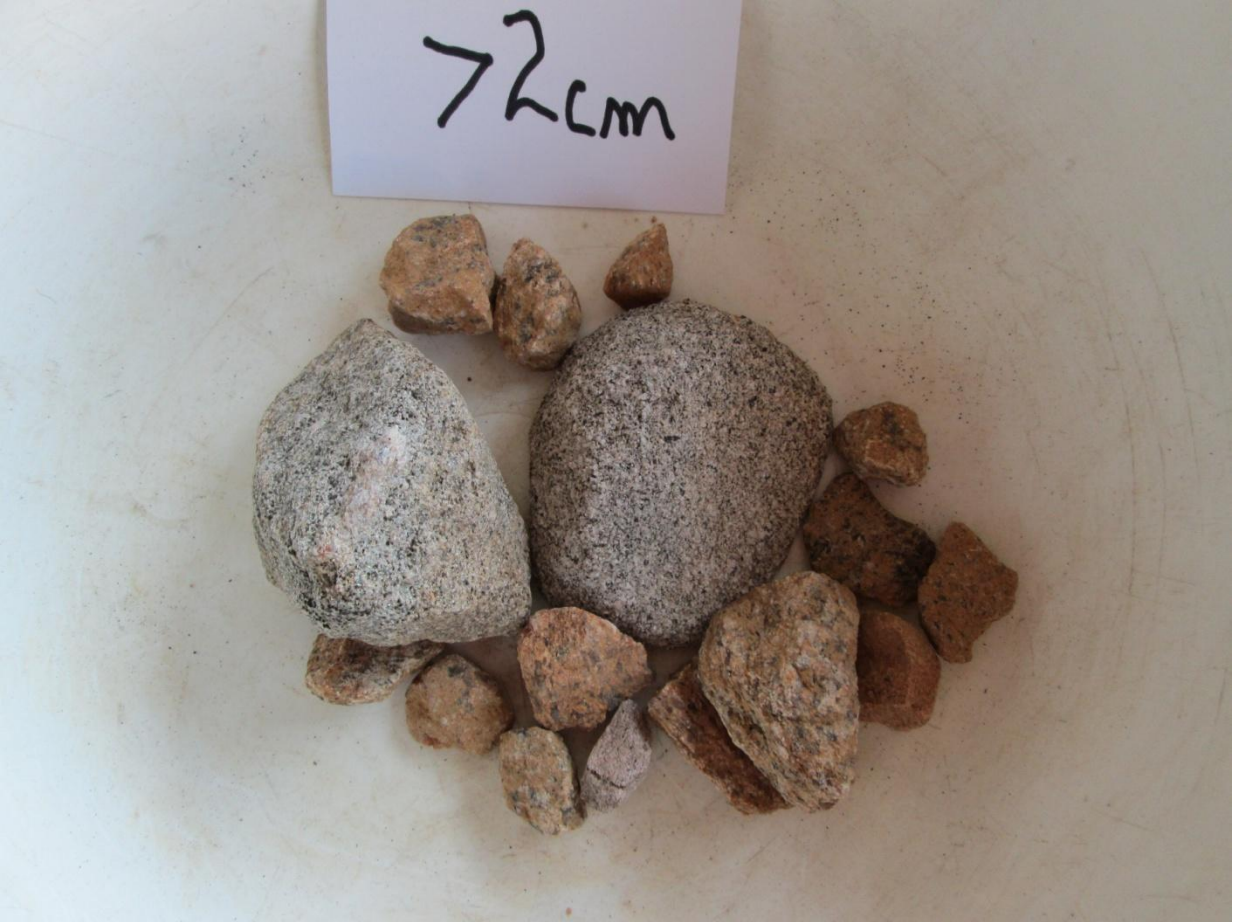
GRAVEL LARGER THAN 2 cm X-SECTION. LARGEST PIECES ARE ABOUT 5cm.
