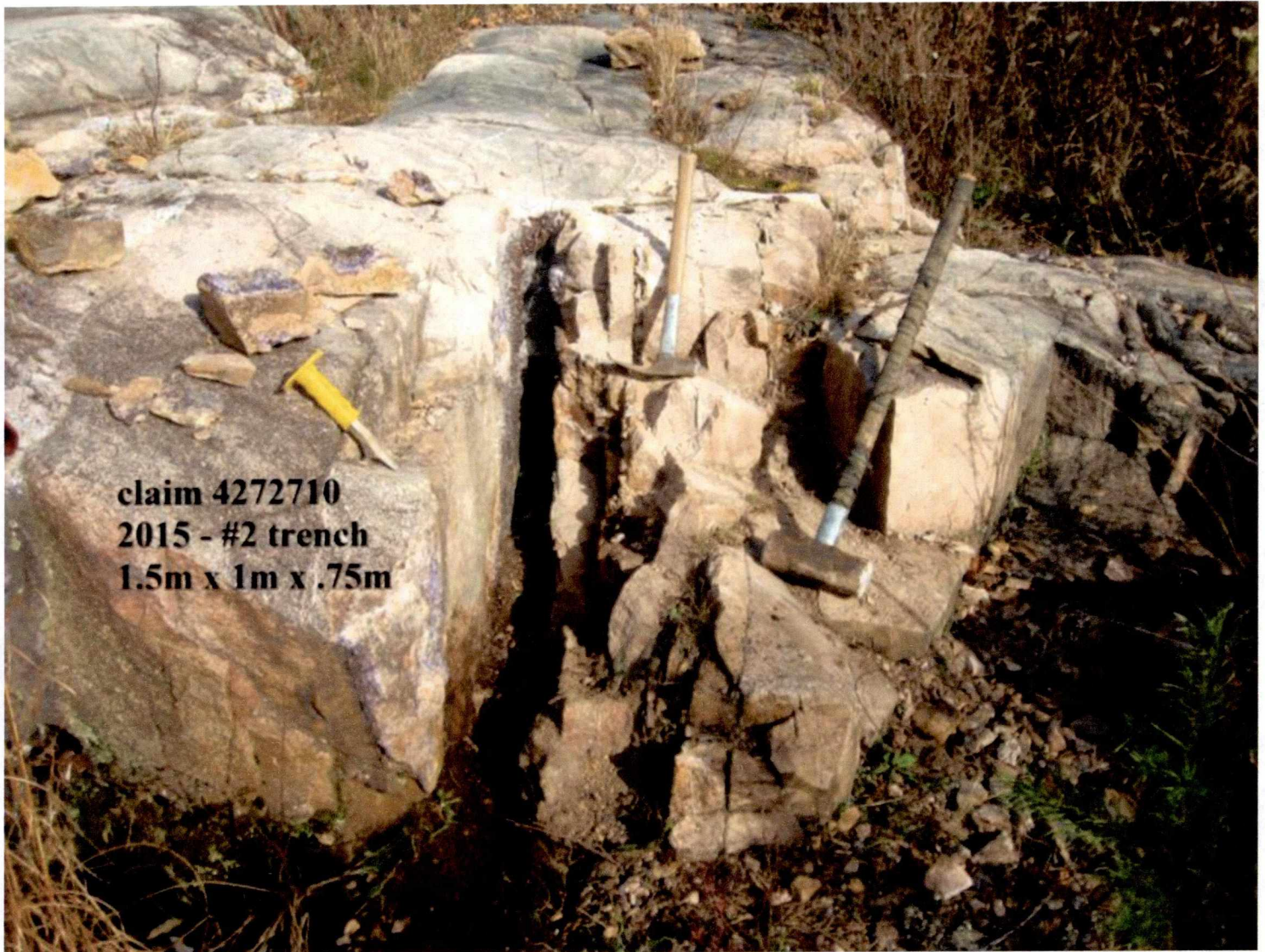
Older trench expanded to approximately 1.5m x 1m x .75m
