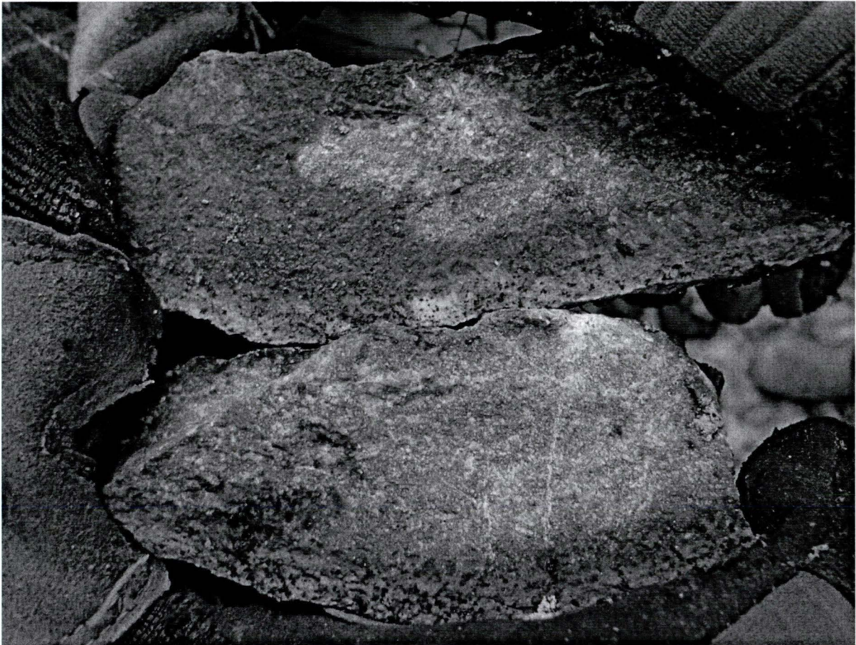
Photo 2: Typical example of carbonate alteration, from mafic unit in contact with porphyry, from west of Zone E
