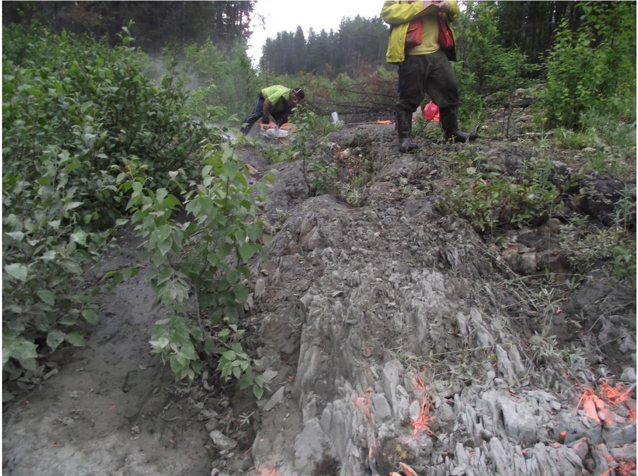
Photo 1: View of shearing at southern exposed end of McKinnon Vein. Shown are channel samples 1409077-82 (bottom) and 1409083-5 (top; being cut)
