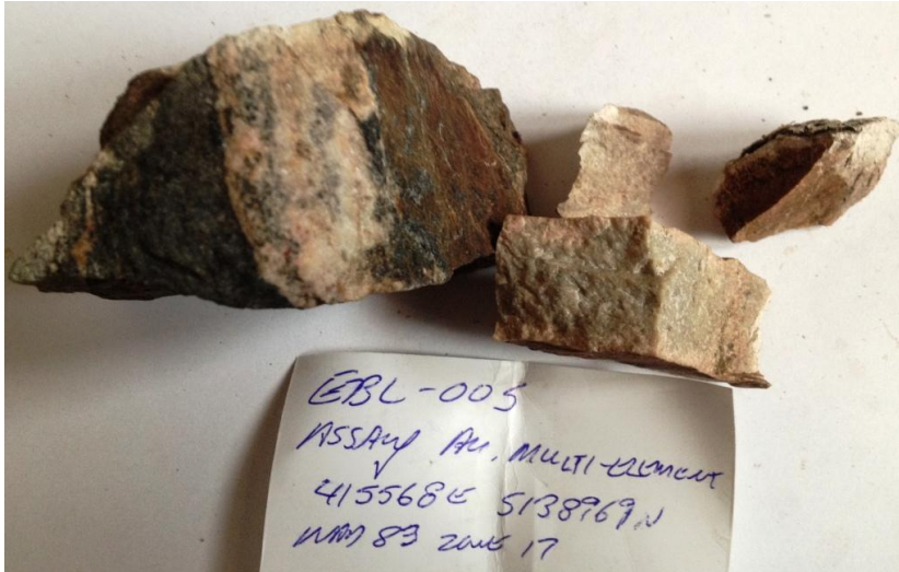
Photo 13: Sample EBL-005, taken from the contact of the syenite and anorthosite. Sample returned anomalous gold and PGE's. Pd and Pt values of 148.4 and 76.4 ppb and 17 ppb Au.
