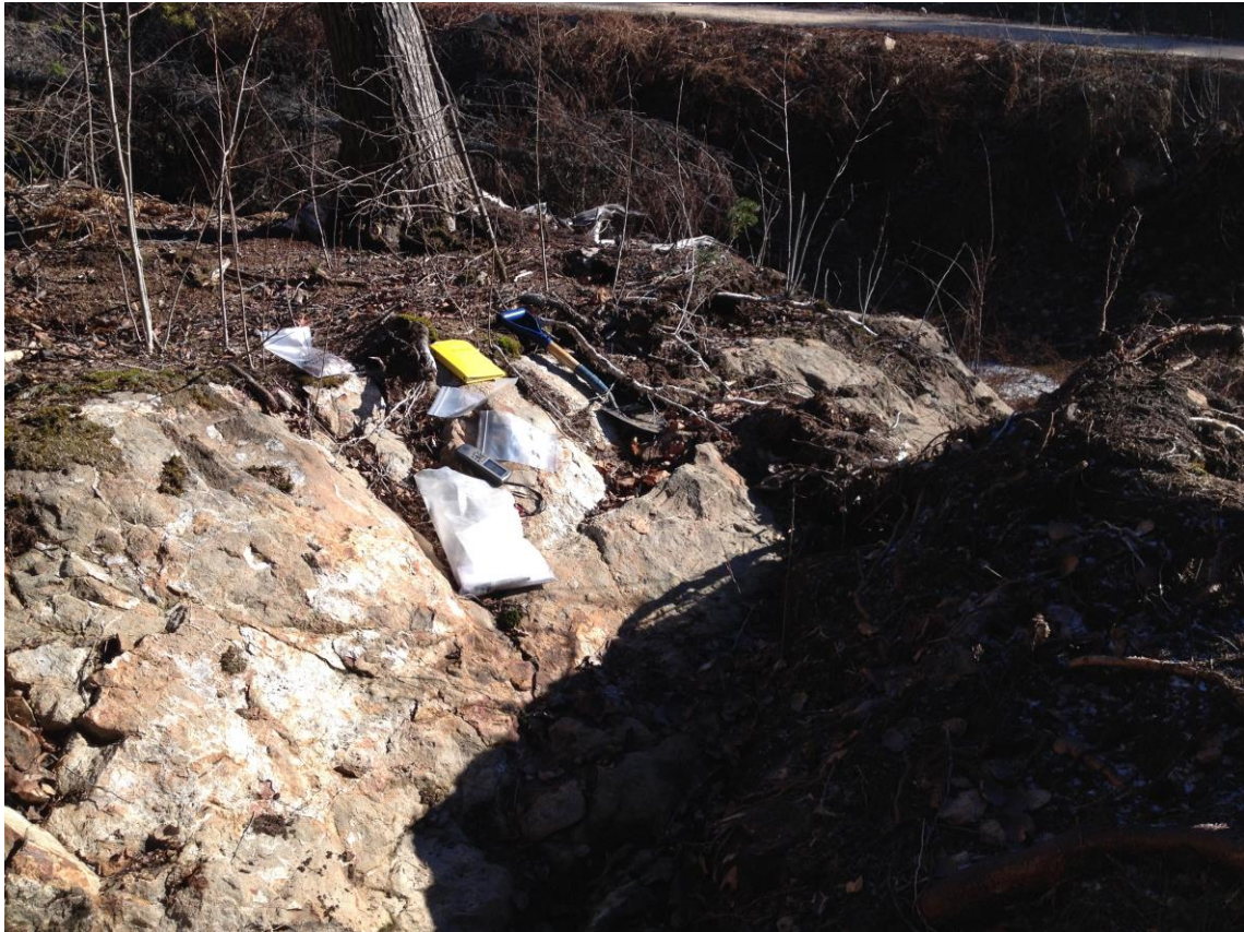
Photo 1: Hand stripping of 2m x 6m rock face area to expose, sample and map the FLDZ
