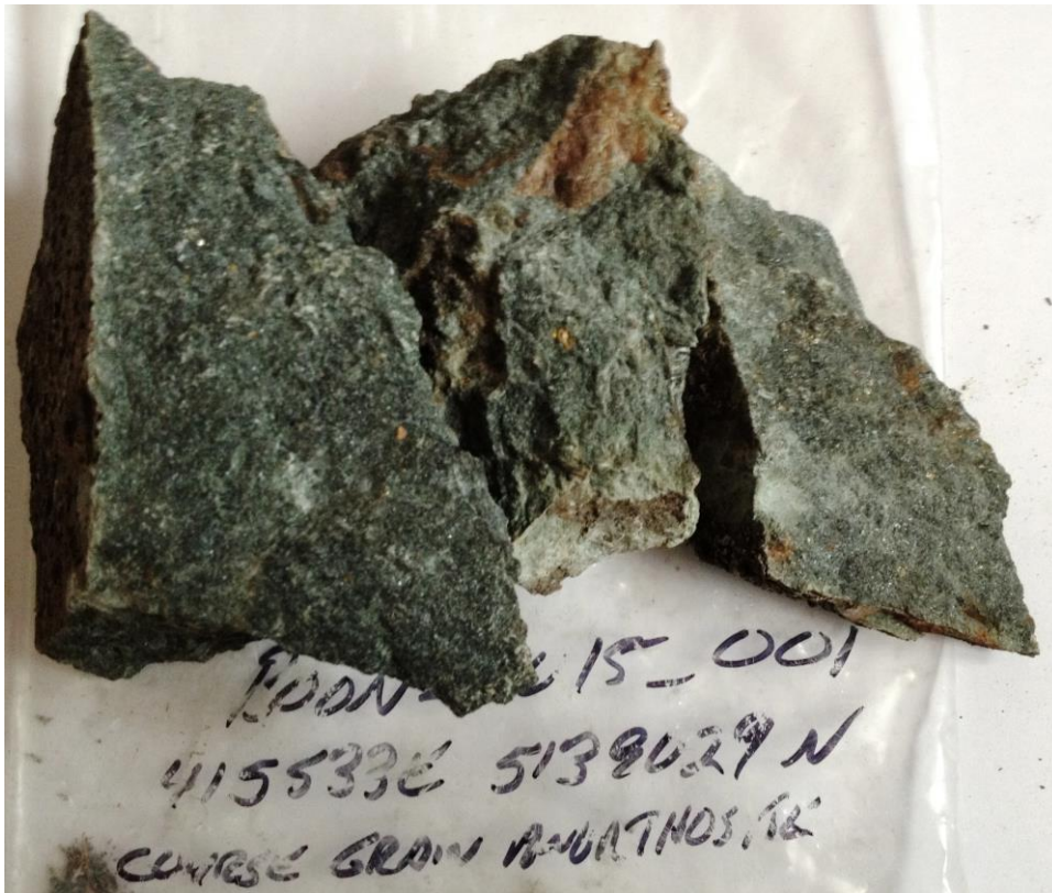
Photo 20: Boon_2015_001, sample of course grained hornblende-gabbronorite with sulfides from magnetic sill area south of road at NAD83 Zone 17 415533 E, 5139029 N. At the time of writing this report the sample has not been submitted for assay.
