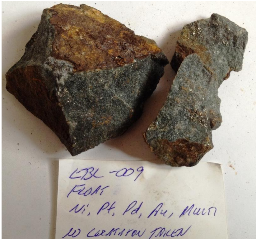
Photo 19: Sample EBL-009, taken from rounded float. Sample contained >5% sulfides so it was assayed to determine the metal sulfide ratios. The results indicated that the greater sulfide content does not necessarily conclude the precious metals will be comparable. Sample returned highest gold of 20 ppb.
