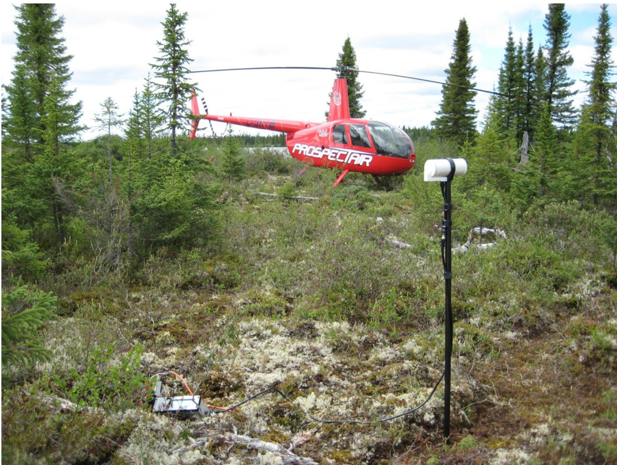
Figure 8: Example of a magnetic base station setup
