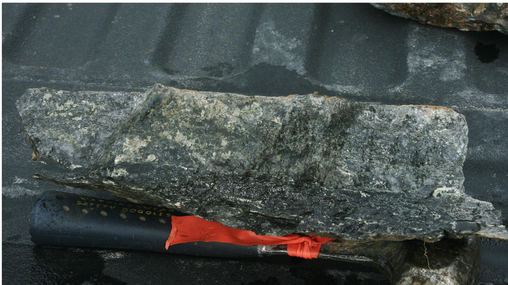
Figure 6. Quartz Vein and Silicified Metasedimentary Rock Mineralized with Pyrite and Arsenopyrite 307792mE, 4964703mN Heron Pond Zone, Black River South Property
