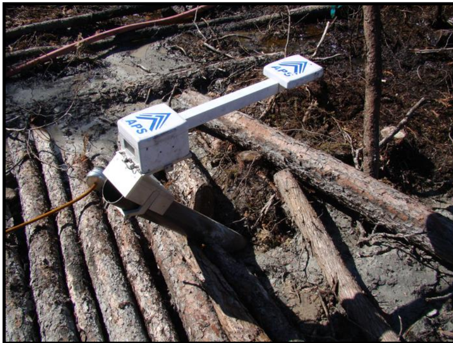
Figure 14: Measuring drill hole collar coordinates, azimuth and dip with a Reflex APS
