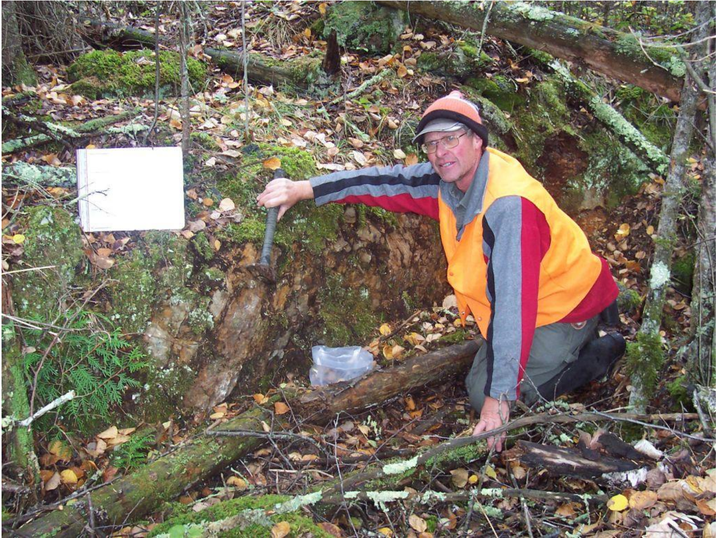
Photo 4. Looking northwest at the author chip sampling trench at 505E/445N in rusty carbonate altered basalt with minor quartz veining (under hammer).
