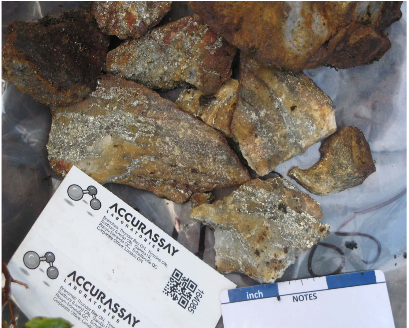
PLA-8) Exhalative Pyritic Cherty Tuff with Banded and Fracture-Fill/In-Situ Breccia Fill Pyrite – Sample 164085 at 5319710N / 615616E
