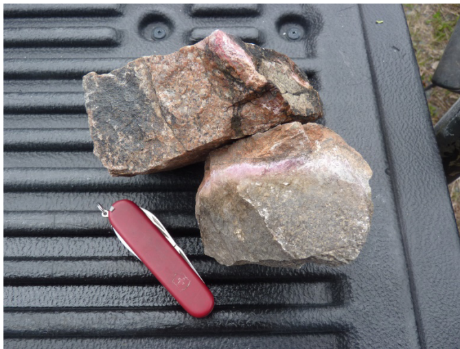
Figure 5 – Cobalt “bloom” in stockpile samples
