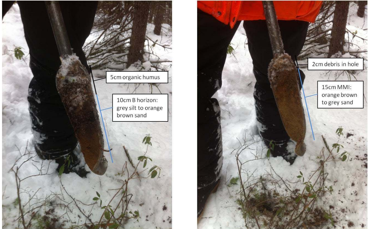
Figure 5: Sampling procedure at a typical 'sandy' site. Ah and B layer samples shown on left, MMI on right. Modified from Brown, 2014.
