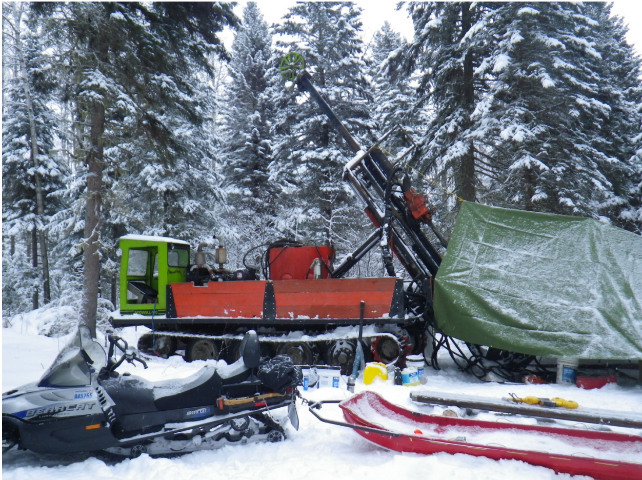
Figure 19. Lavoie home-built Nodwell mounted diamond drill on 16ER01 collar site.
