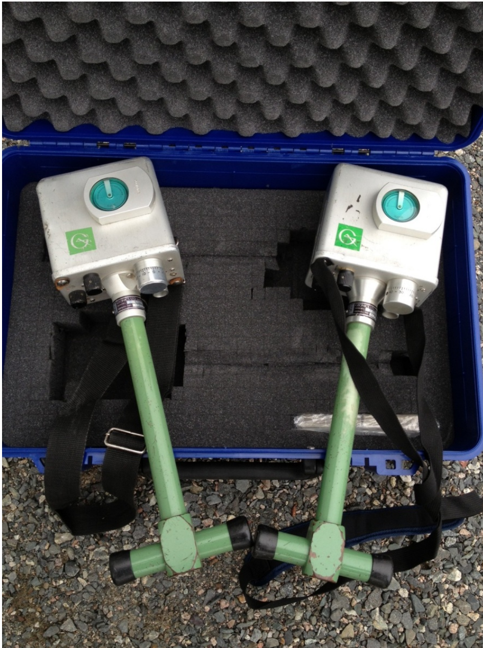
Figure 9: Geonics EM-16 VLF Instruments used at Eric Lake.
