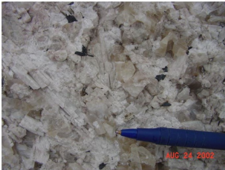
Figure 7-7 Black manganocolumbite-manganotantalite in spodumene-rich zone of the Main Dyke (Breaks et al., 2006, OFR 6195).
