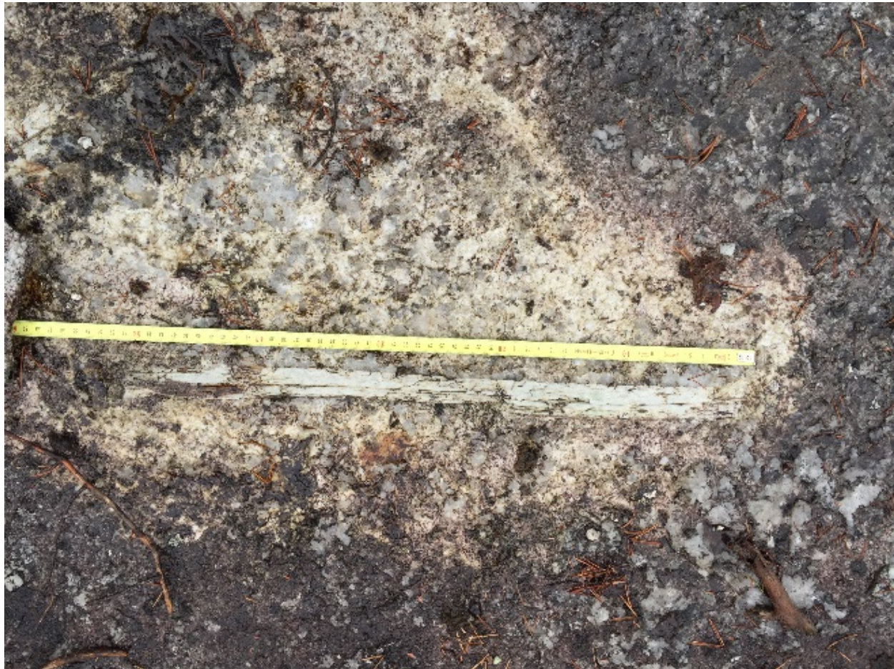
Figure 14-9 A 53 cm long spodumene crystal in a matrix of coarse-grained spodumene + grey quartz from North Dyke
