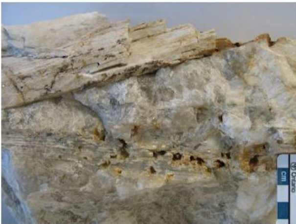
Figure 7-6 Spodumene megacrysts, quartz and white K-feldspar from Main Dyke (Breaks et al., 2006, OFR 6195). Rusty pock marks in the spodumene represent weathered sphalerite.
