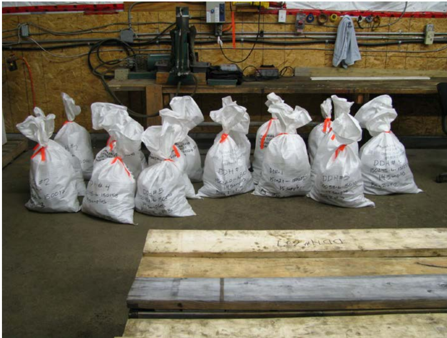
Figure 11-1 Sealed rice bags labelled with drill hole number and sample range.
