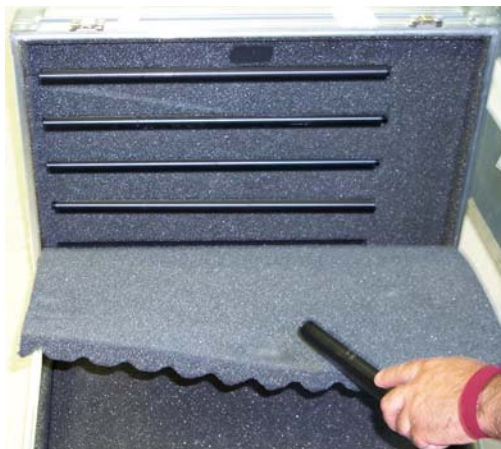
Figure 2. GSM-19 Case with Sectional Staff rods. Assemble these rods if you are planning to conduct a “Mobile” survey (i.e. one with discrete stations as opposed to a “walking” or continuous survey).
