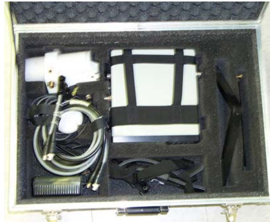
Figure 3: Standard magnetometer components include a sensor, console, radio frequency cable, download cable, shoulder harness, sensor mounting rod, and RS-232 cable. Also included here are a GPS and GPS support rod. For a complete list of parts, consult your packing slip. It may show, for example, that you have an additional sensor and radio frequency cable (i.e. for a gradiometer configuration).
