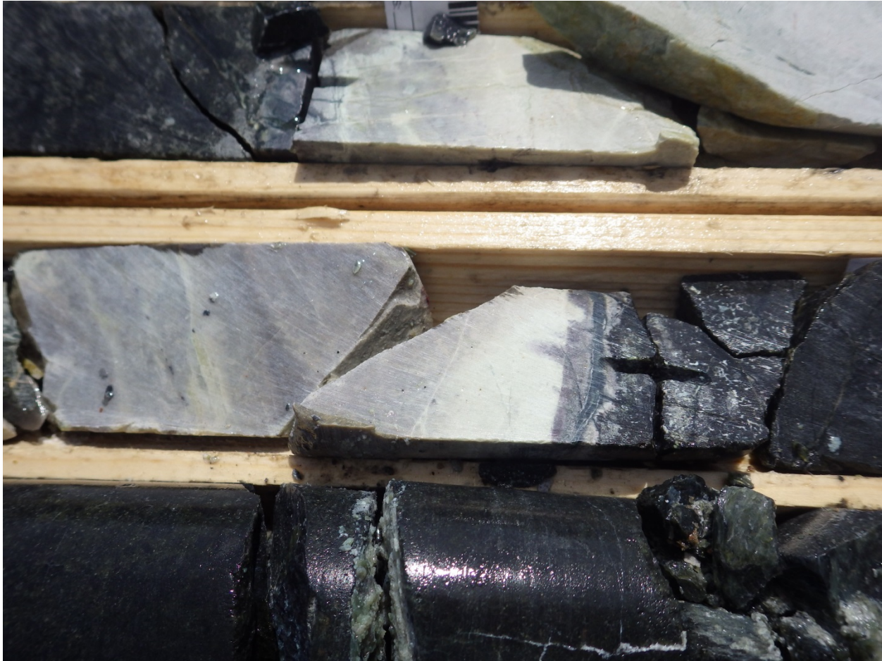
Photo 1. Silicified dacite overprinted by quartz veining and Clay Alteration at 20.47m (sample L782755) downhole from hole MD-17-001
