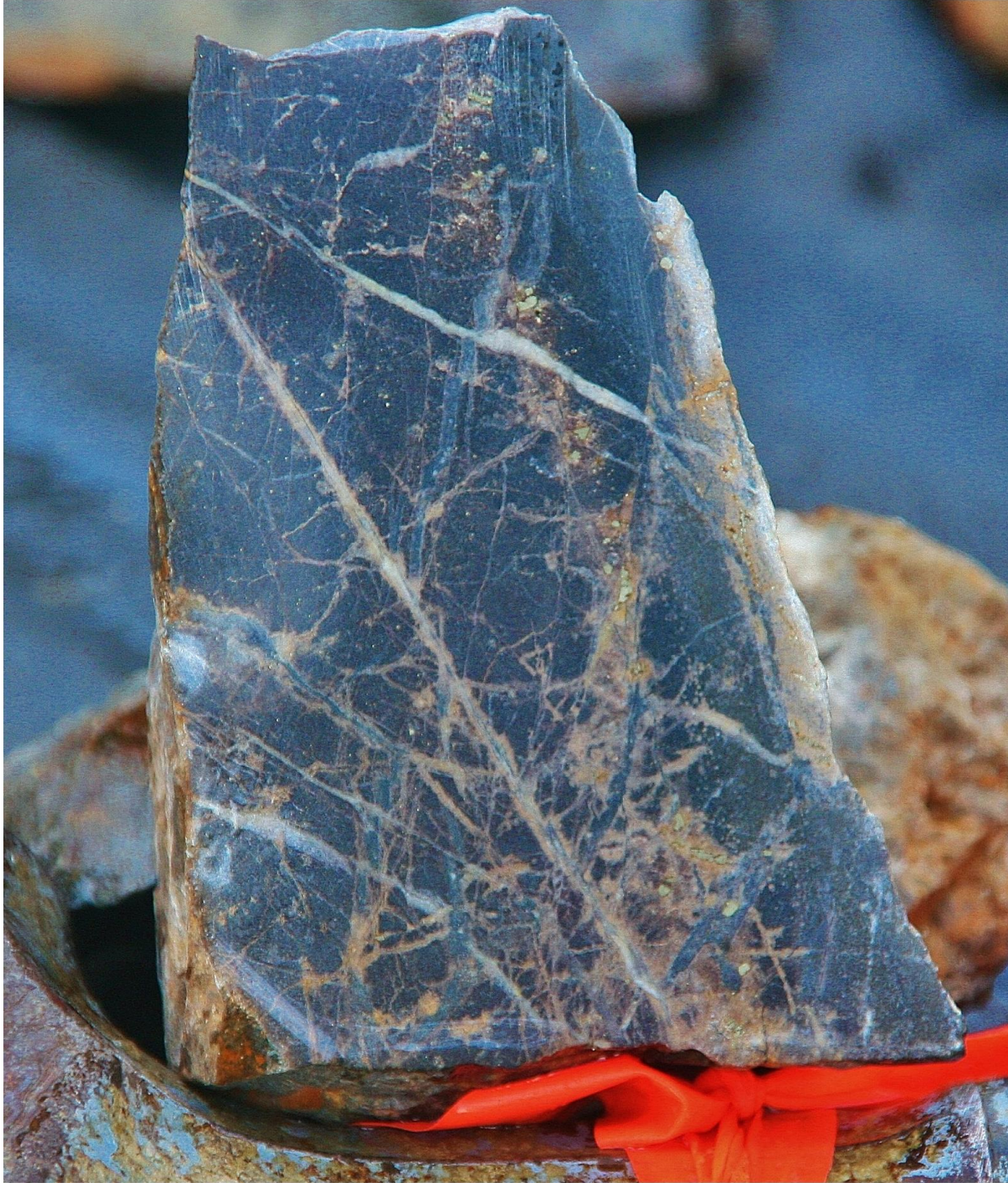
Figure 12: Magusi Trench, quartz-carbonate stringers and fracture-filling with pyrite and hematite. Note the crosscutting white calcite stringers. Tannahill-Holloway Twp's., Ontario
