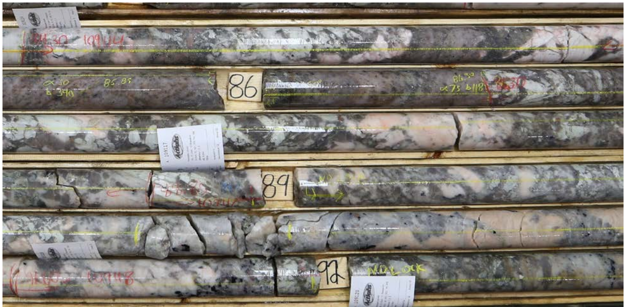
Photo 3: Core photo highlighting sampling procedures (red crayon) and captured core orientation measurements (yellow)
