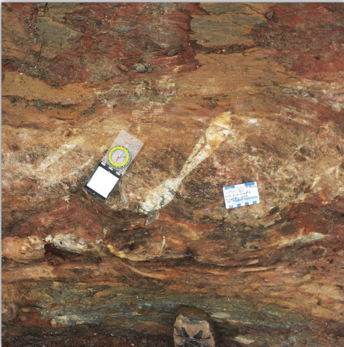
Figure 19 - Late quartz veining cross-cutting a mineralized quartz vein boudin in the McKellar Pits area.
