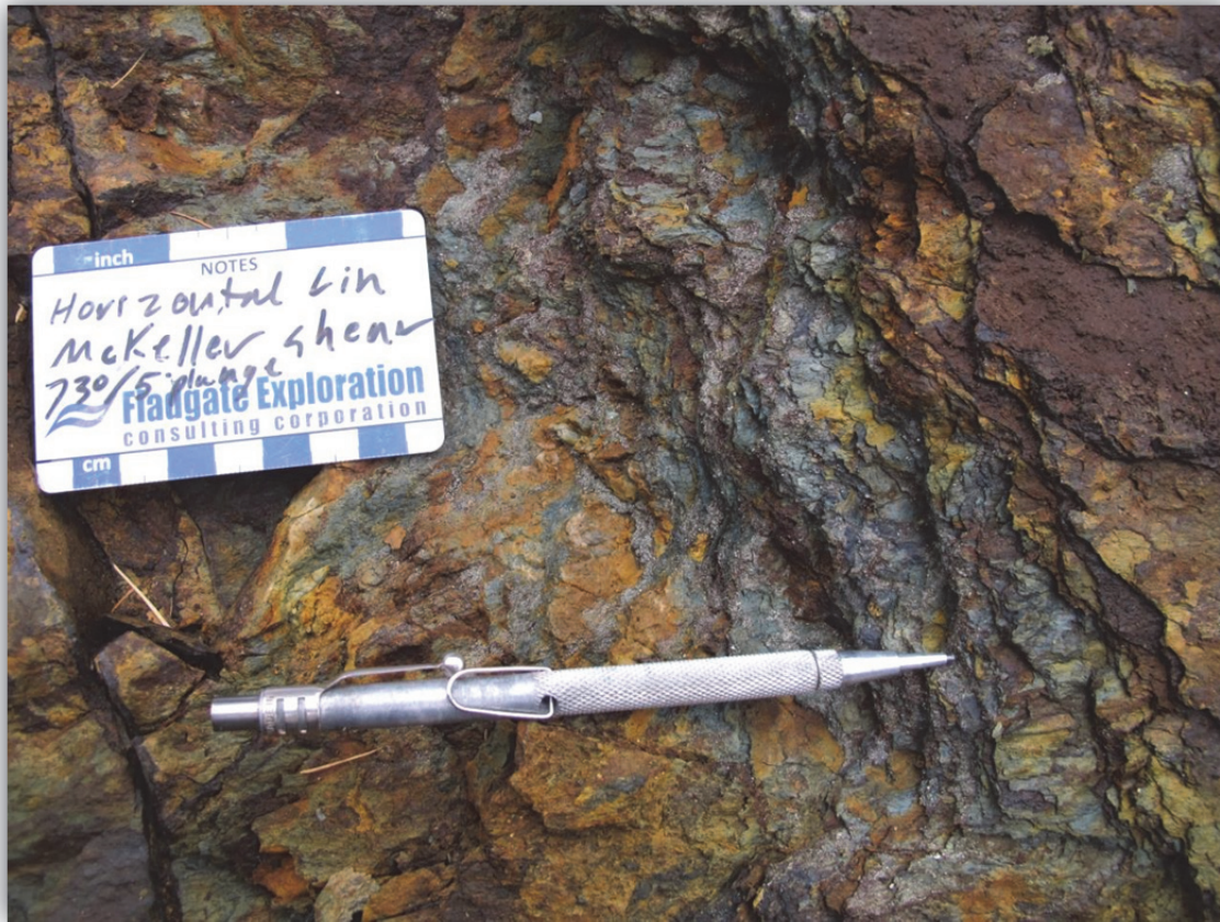
Figure 15 - Strong horizontal ( 73^{\circ}/5^{\circ} ) stretching lineations in the McKellar shear parallel to the pervasive mineral lineation.
