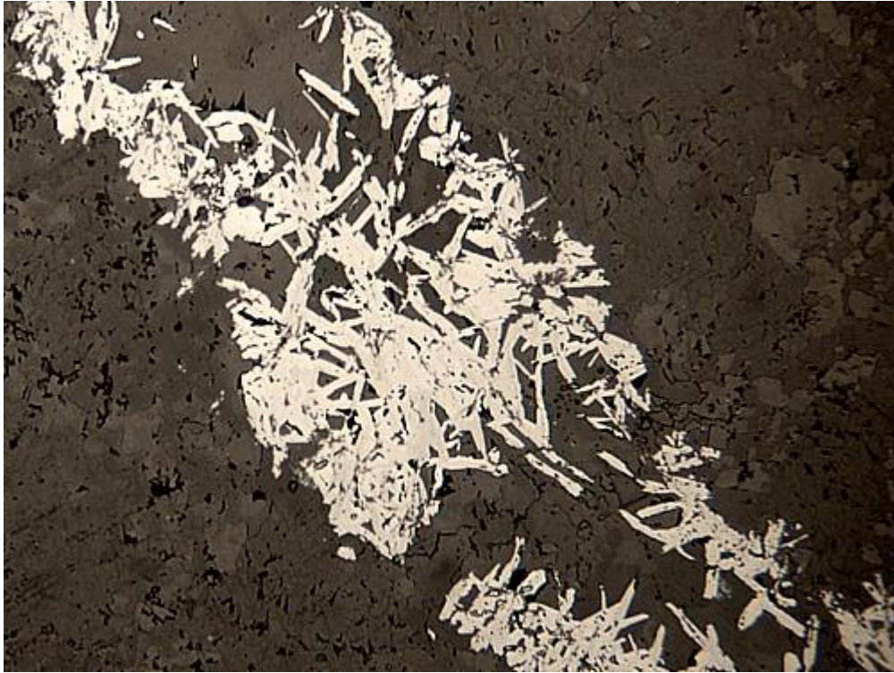
Specular hematite vein. X-axis of photo: 0.64mm. Refl. light.
