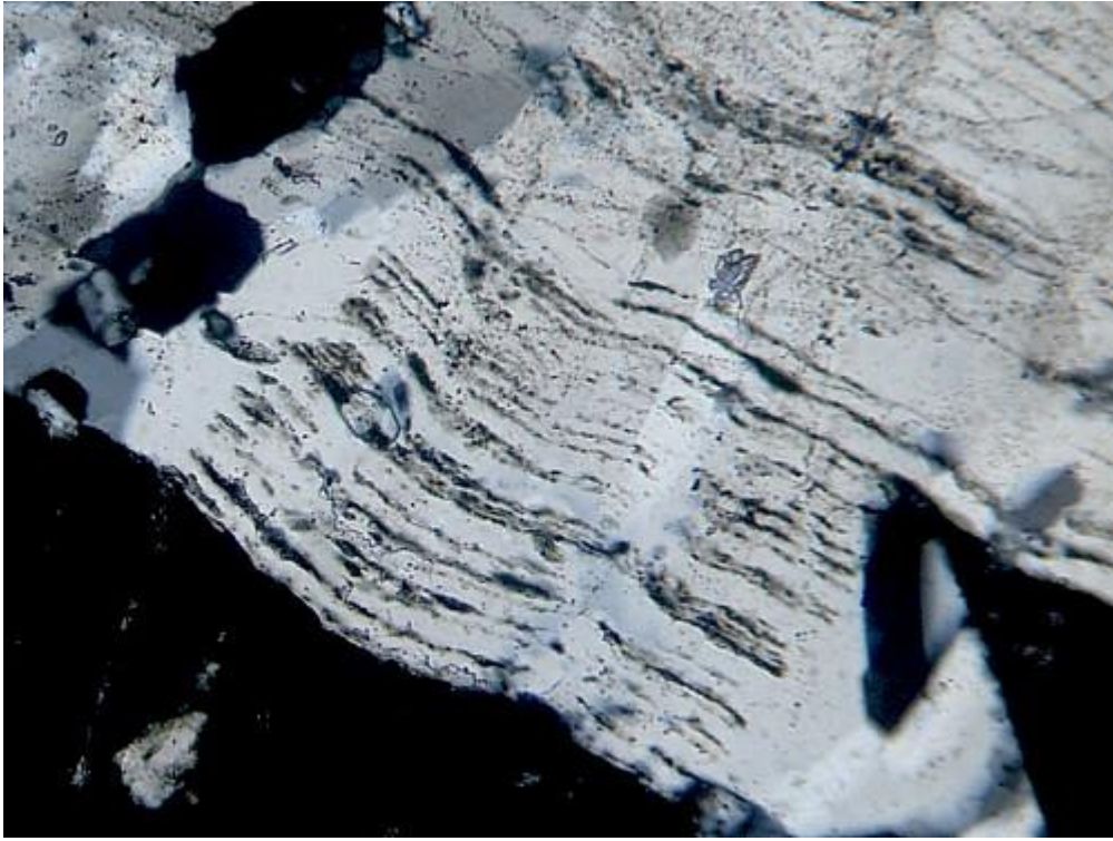
Sheared and deformed vein quartz. X-axis of photo:0.64mm. XN.
