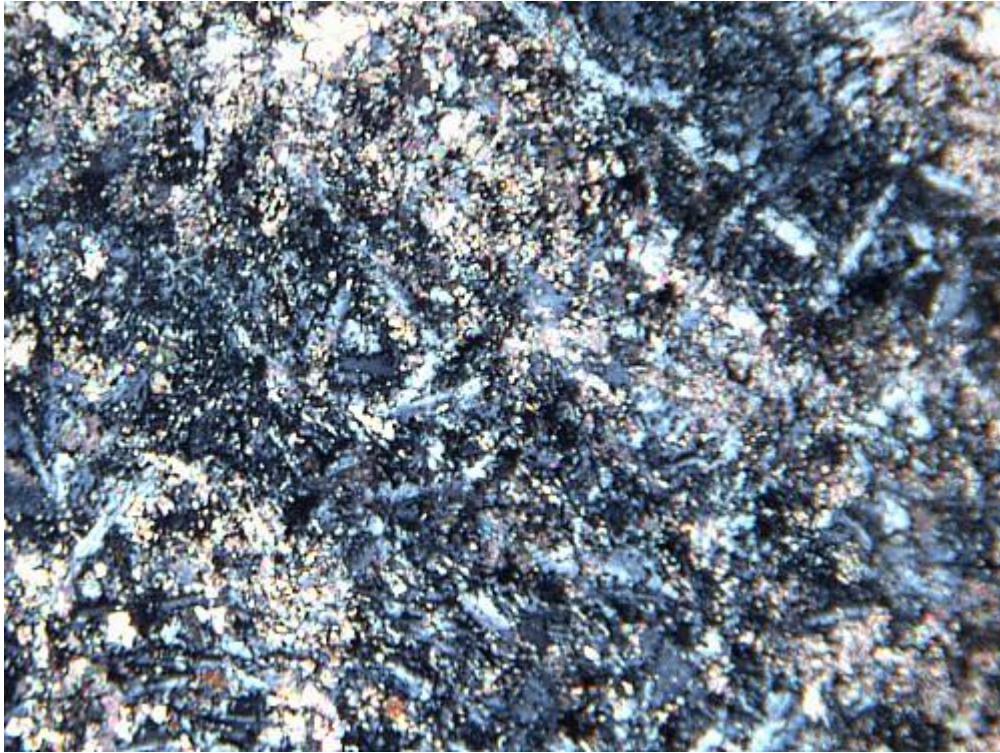
Relict volcanic texture with interstitial fine-grained carbonate. X-axis of photo: 1.6mm. XN.
