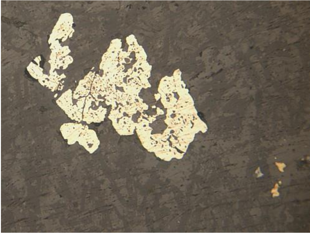
Anhedral pyrite in andesite. X-axis of photo: 0.64mm. Refl. light.
