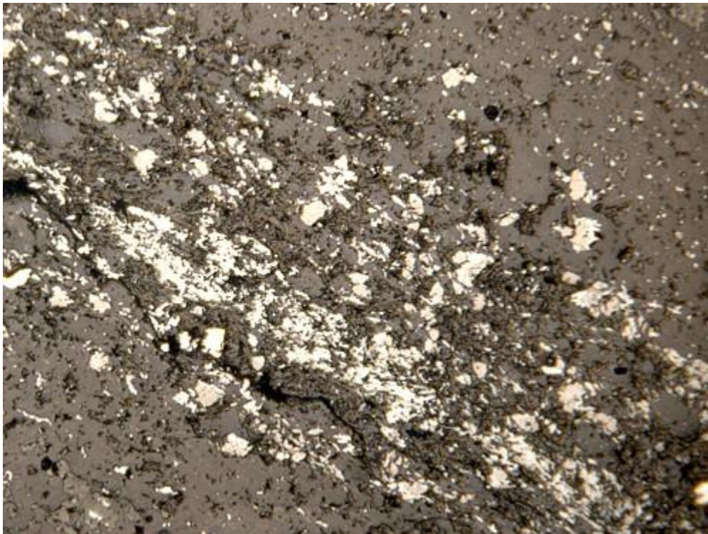
Fine-grained hematite + pyrite vein (in carbonate-rich matrix). X-axis of photo: 1.6mm. Refl. light.
