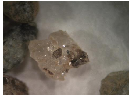
21. 1.2mm – Fractured with mica inclusions
