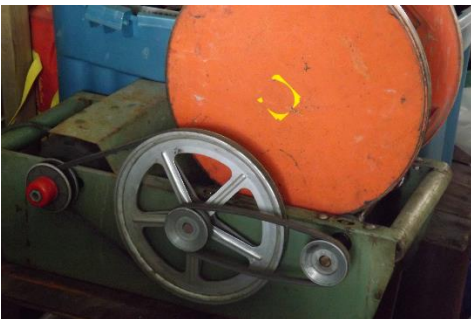
4 - Variable speed industrial tumbler
