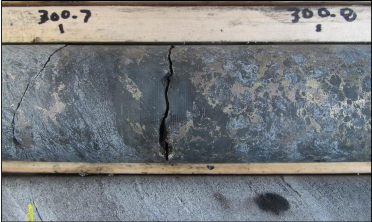
Plate 3: Black, fine-grained tourmalinite-rich section of the massive sulphide horizon.
