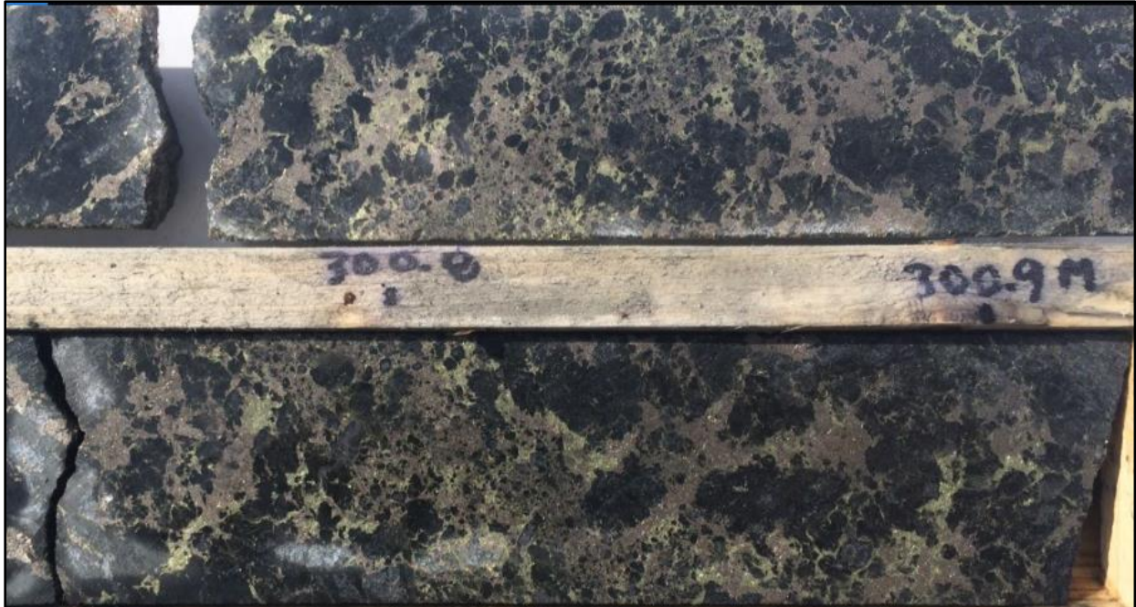
Plate 1: High grade portions of the massive sulphide horizon. (metre marks refer to core in lower row, Sample 390032. Upper row is part of sample #390029)
