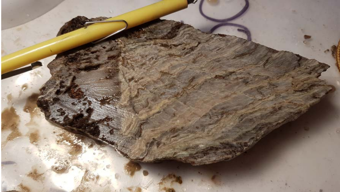
Figure 4. Channel sample from Trench #3, 2017 trenching exhibiting strong sericite/silicification/carb alteration, strong shearing with crenulation cleavage, cut by a fairly fresh, vuggy quartz vein.
