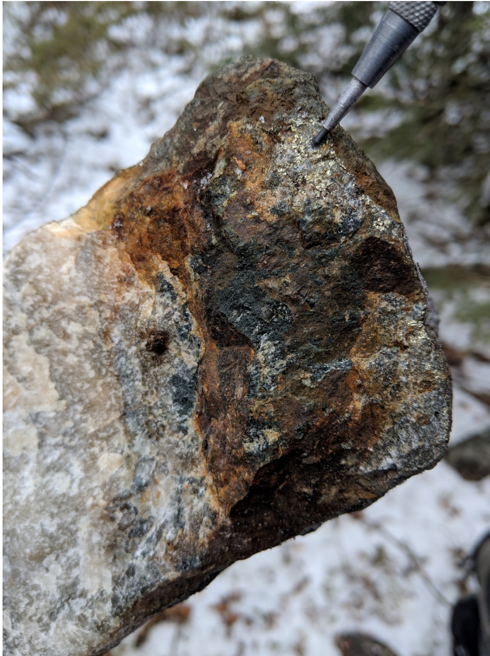
Figure 8.2: 2018 Sample # 3216859 taken from Black Jack, showing quartz veining and sulfidation in vein selvage. Assay results returned 2.815 ppm Au and 2995.3 ppm Cu.
