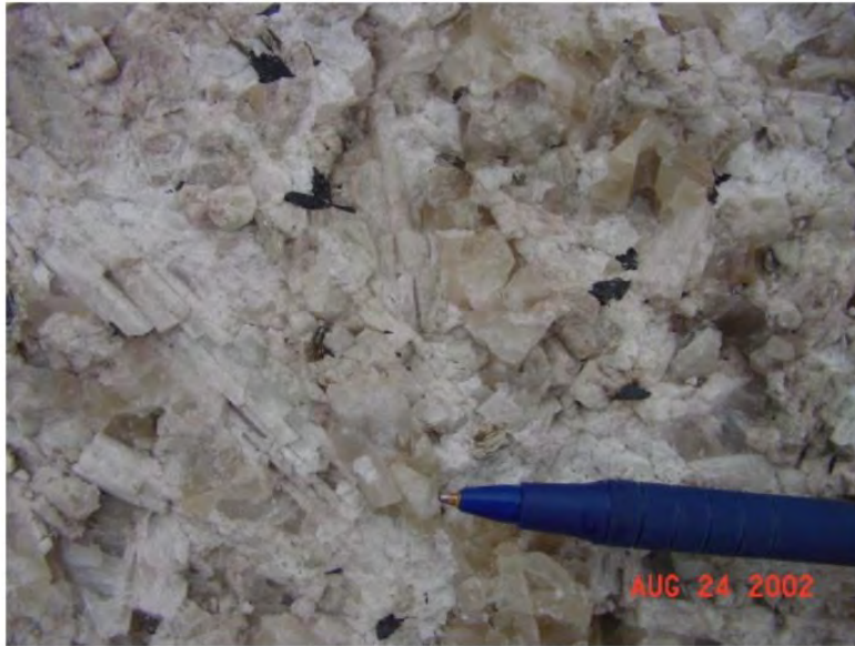
Figure 7-8 Black manganocolumbite-manganotantalite in spodumene-rich zone of the Main Dyke (Breaks et al., 2006, OFR 6195).
