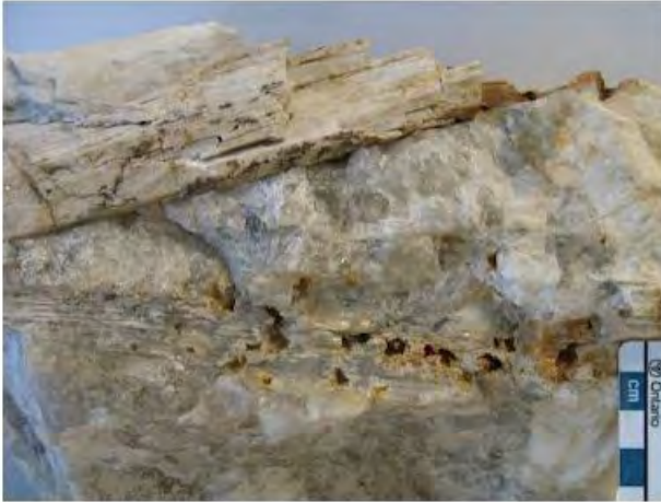
Figure 7-7 Spodumene megacrysts, quartz and white K-feldspar from Main Dyke (Breaks et al., 2006, OFR 6195). Rusty pock marks in the spodumene represent weathered sphalerite.
