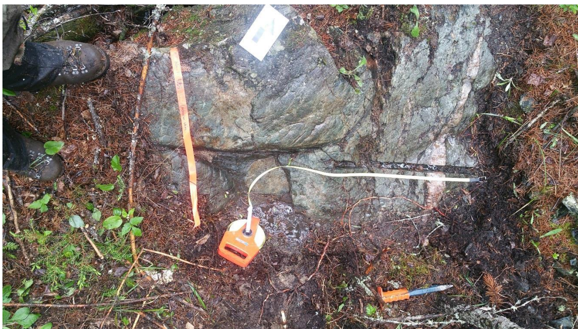
Figure 9.7: Locating and taking a representative sample of 1986 channel sample number 4703 of the Combination Vein.
