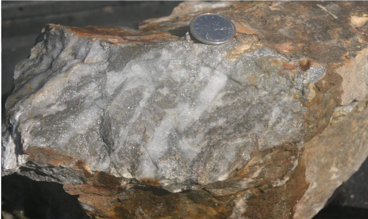
Figure 33. Trench-2 Quartz with fragments of greywacke and arsenopyrite. Sample TR-12 Trench debris 357917mE, 5495232mN
