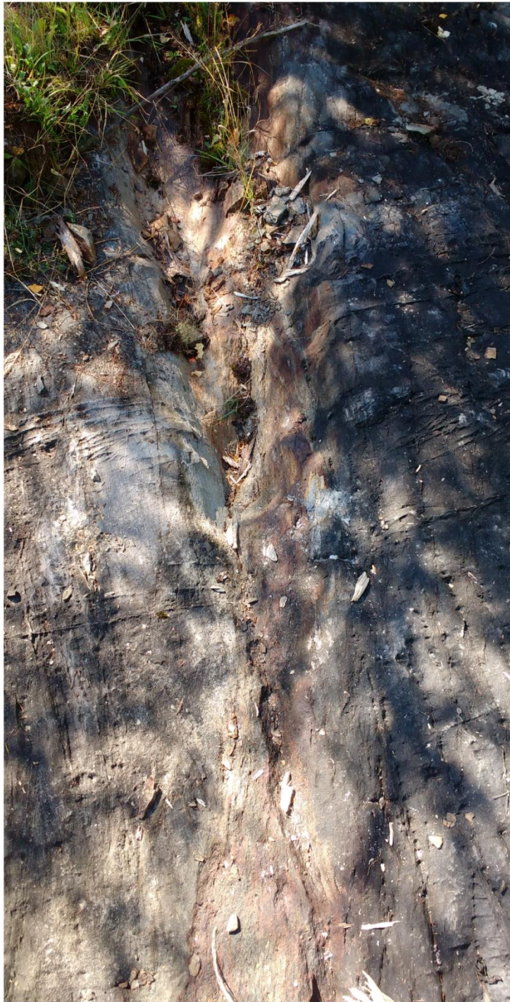
Figure 13. Outcrop in ditch east side of McCowan Road Pyrite bearing quartz stringer stockwork in greywacke 358611mE, 5495847mN Looking west Rock sample location TR-19, TR-20 & TR-21
