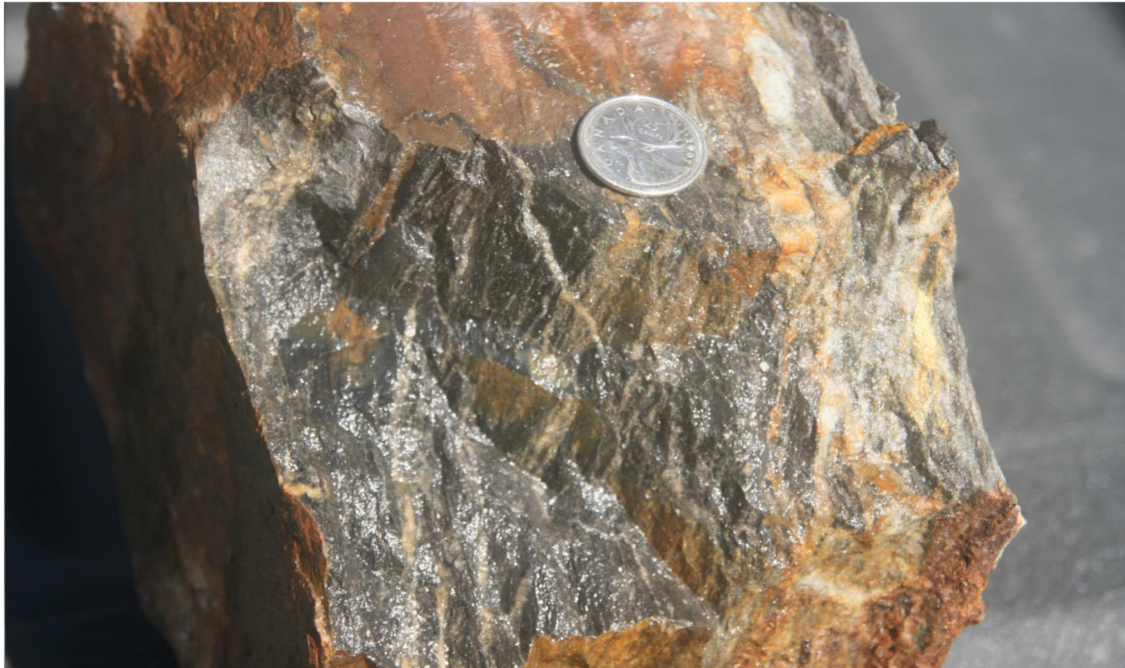
Figure 32. Trench-2 Silicified Greywacke with quartz and arsenopyrite adjacent quartz vein. Trench debris. Sample TR-11 357957mE, 5495241mN
