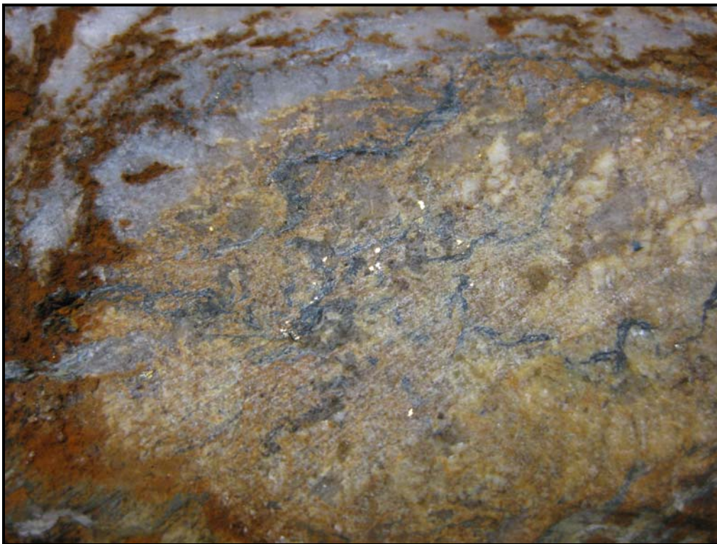
Plate 4: Gold grains in high-grade quartz/carbonate veining from Flint Lake Mine
