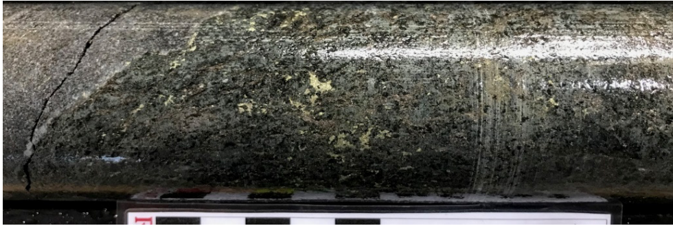
Figure 7: Core photo of QTBL0005 at 20.9m, showing recrystallized Chl-Bt-Cpx ultramafic unit with interstitial chalcopyrite in contact with meta-sediment
