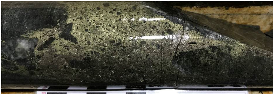
Figure 17: Core photo of QTBL0009 at 50.8m showing massive chalcopyrite-pyrrhotite forming a thin breccia at low-angle to core axis, with sub-rounded inclusions of the host paragneiss.
