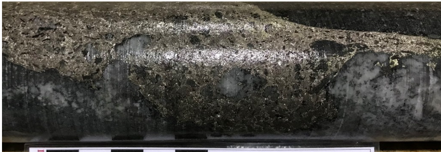
Figure 16: Core photo of QTBL0009 at 50.6m showing massive pyrrhotite-chalcopyrite forming a thin breccia at low-angle to core axis, with sub-rounded inclusions of the host paragneiss.
