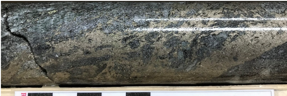
Figure 8: Core photo of QTBL0005 at 21.8m, showing recrystallized showing a thin interval of semi-massive sulphides (pyrrhotite-pentlandite) where sulphides form the matrix of a brittle-ductile shear zone within gneissic meta-sediments.
