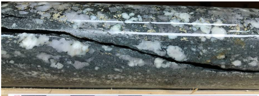
Figure 18: Core photo of QTBL0009 at 146m showing a brecciated pegmatite within paragneiss. The fault breccia is at low-angle to core axis and has a matrix of chlorite-biotite-pyrite.
