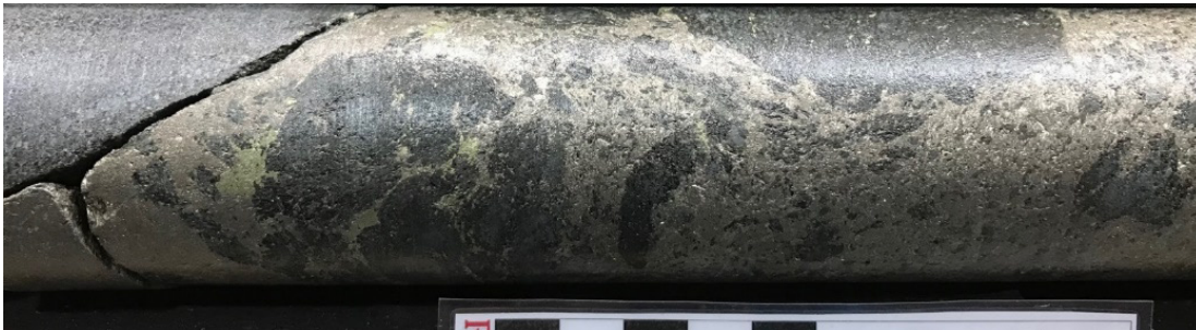
Figure 9: Core photo of QTBL0005 at 22.9m showing the upper contact of the massive sulphide unit (pyrrhotite-pentlandite-chalcopyrite) with cm-size inclusions from the host meta-sediments.
