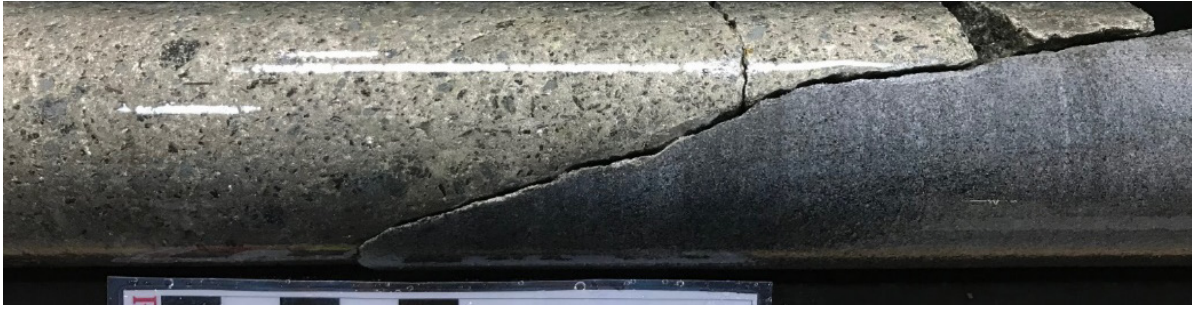
Figure 11: Core photo of QTBL0005 at 23.8m showing the lower contact of the massive sulphides unit in contact with meta-sediment.
