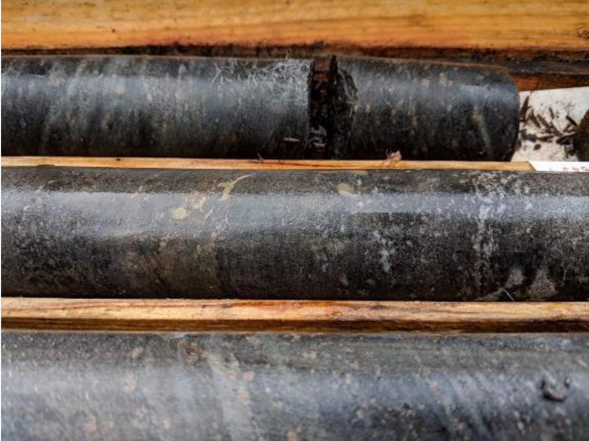
Photo: Disseminated sulphides in historical drill core
