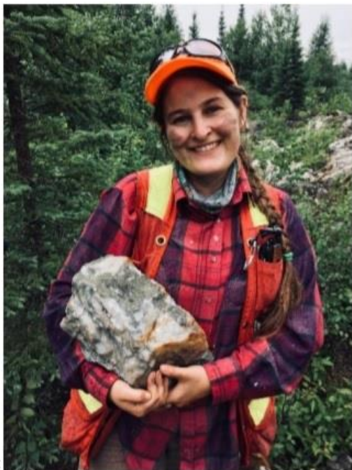
Figure 1 . a) Contact between chlorite schist and highly fractured quartz vein at the Minto North occurrence (looking northeast). b) Tension veins indicating sinistral movement. c) RGP District Geological Assistant S. Hinz holding sample with pyrite stringers hosted by quartz. Grab sample from this location returned 1.3g/t Au. d) Sulphide patches and burns in the highly fractured quartz vein.
