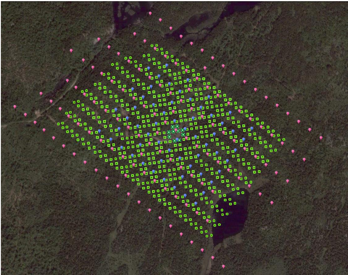
Figure 3: Survey Design Model Looking Down – Red=Current Injection, Blue=Receiver Electrodes, Green=Theoretical Data Point (©2018 Google, Image ©2018 DigitalGlobe)
