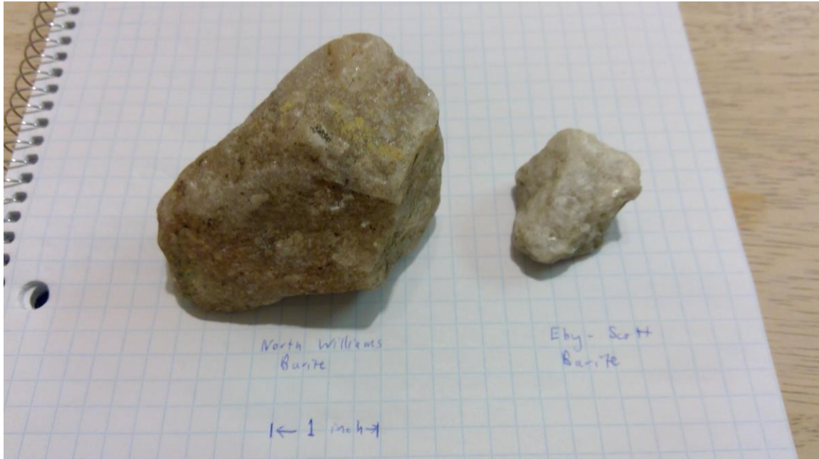
Figure 2: Barite samples from North Williams township (Extender Minerals mine), Left, compared to Lawson Twp Eby Scott deposit, right. Note clean white colour of barite from Lawson township.
