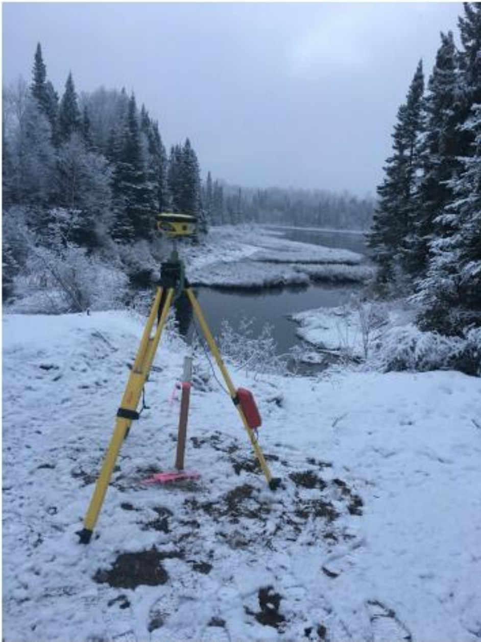
Figure 4 – RME Geomatics BASE station deployed during the Jackpot Mine survey.
