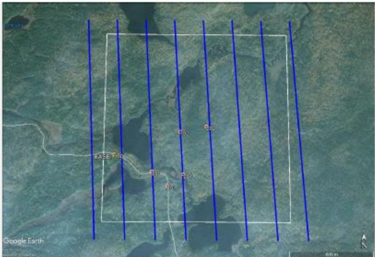
Figure 1 - Jackpot Mine area flight lines (blue), area of interest (white), GCPs (red/white markers), and BASE monument (green triangle) overlain on Google Earth imagery.
