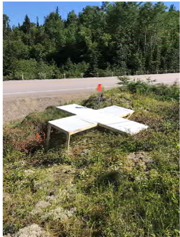
Figure 5: White crosses marking the four geodetic stations clockwise from the top left corner - 0011993U226, 0011993U367, 0011993U366 and 0011993U368.
