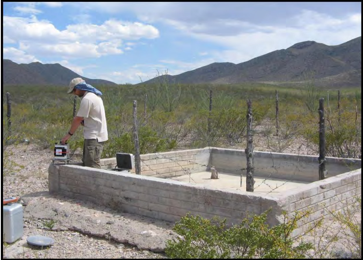
Figure 11. The single ground control point used to reference the 260 km 2 stereo WorldView-1 elevation mapping project in Chihuahua, Mexico.
