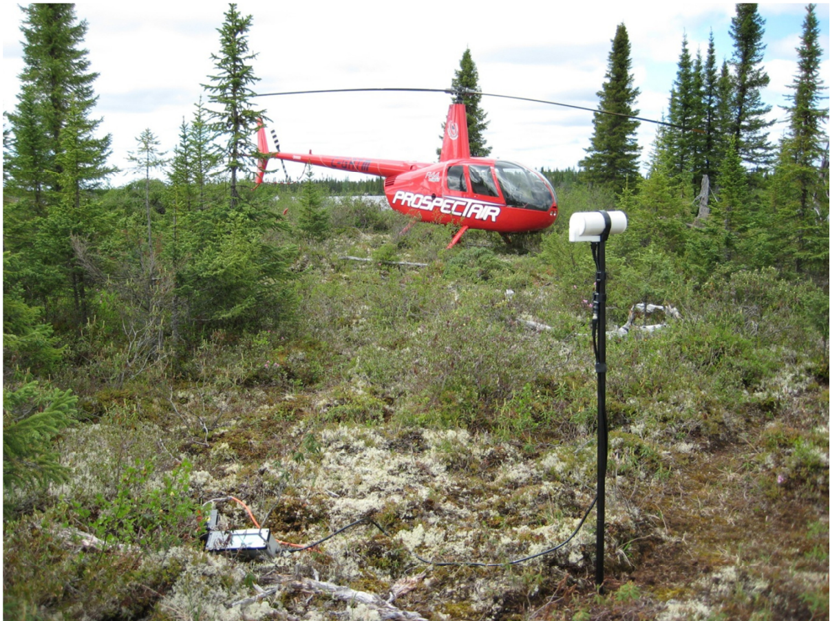
Figure 5: Example of a magnetic base station setup
