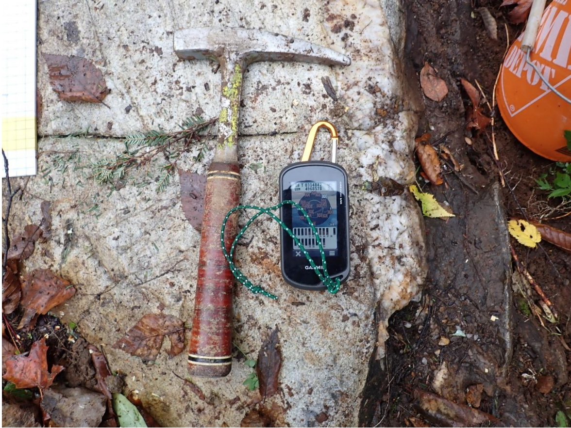
Figure 19: Outcrop 16 of Trench Map 1, Quartz Porphyry with 5-10cm thick quartz veins, hammer for scale: 33cm.
