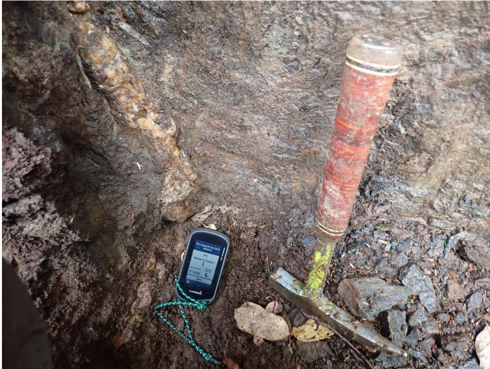
Figure 11: Outcrop 8 of Trench Map 1, Mafic Dike with steeply dipping quartz veins (Unit 3abce MNDM Map Easton 2001), 60.3g/t, 40.3g/t, and 17.9g/t Au assay results, hammer for scale: 33cm
