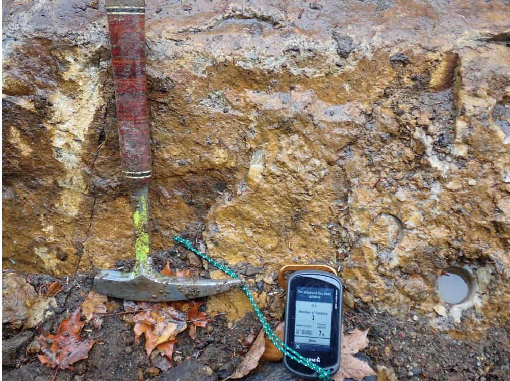
Figure 12: Outcrop 9 of Trench Map 1, Quartz Porphyry with shallow dipping quartz veins, hammer for scale: 33cm.
