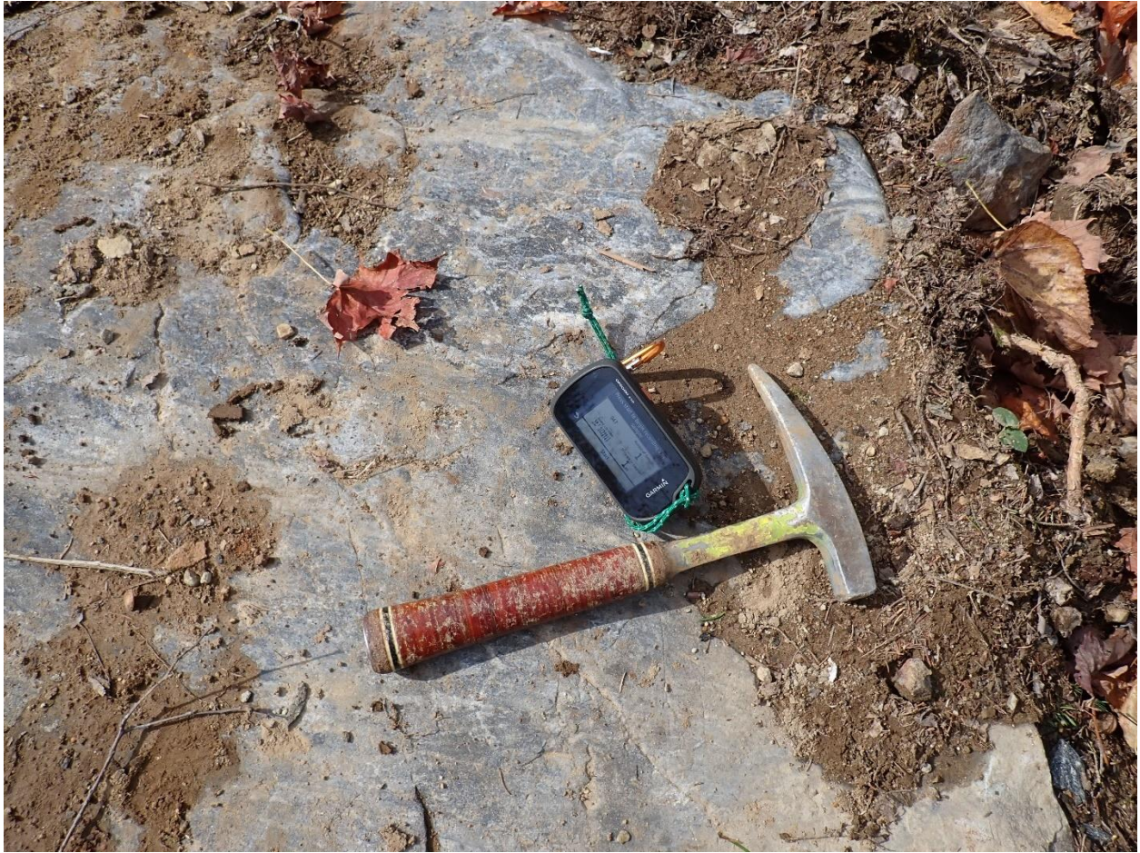
Figure 35: Outcrop 15 of Trench Map 2, Iron Formation with quartz veins showing sugary texture within fresh surface, hammer for scale: 33cm.
