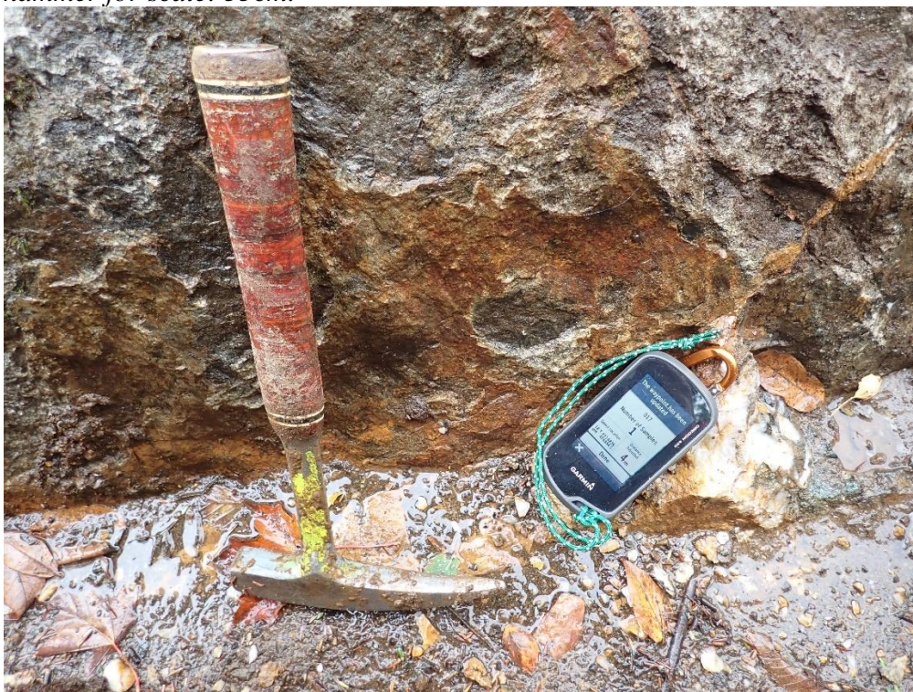
Figure 14: Outcrop 11 of Trench Map 1, Quartz Porphyry with shallow-dipping quartz veins, hammer for scale: 33cm.
