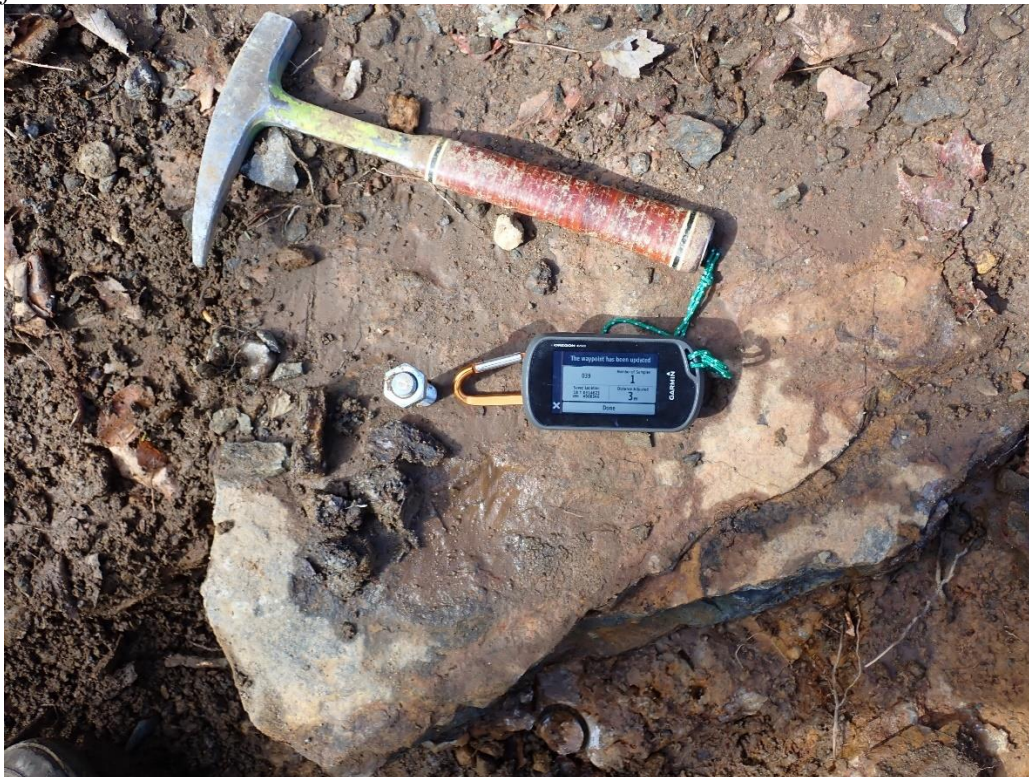
Figure 26: Outcrop 6 of Trench Map 2, Iron Formation with chloritized quartz veins, hammer for scale: 33cm.
