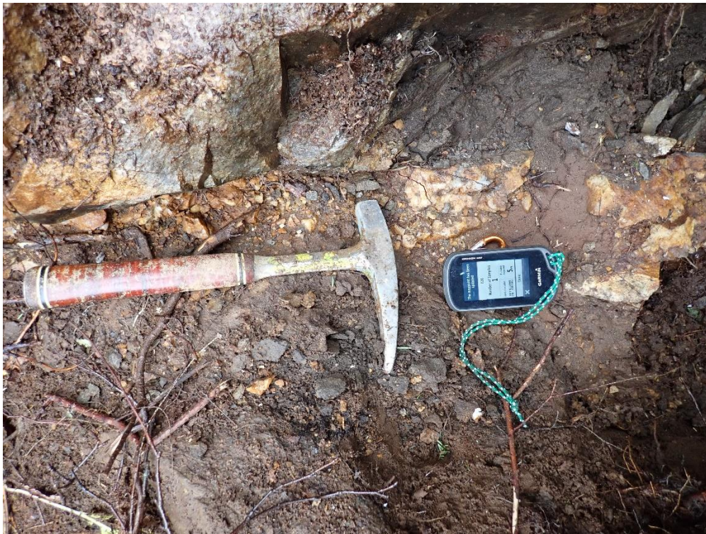
Figure 18: Outcrop 15 of Trench Map 1, Quartz Porphyry with approximately 5-10cm thick quartz veins, hammer for scale: 33cm.
