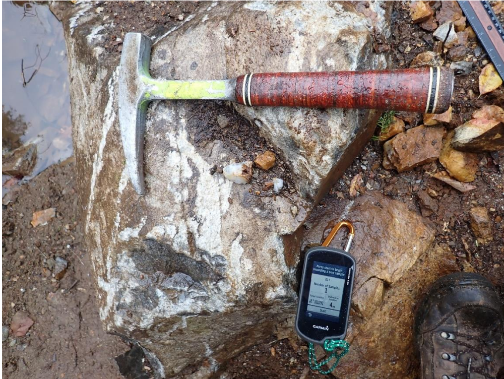
Figure 7: Outcrop 4 of Trench Map 1, Quartz Porphyry with quartz veins, hammer for scale: 33cm.
