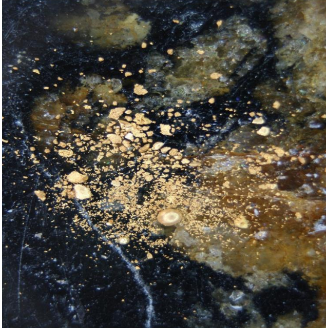
Figure 39: Gold hand concentrated from 2kg of quartz from the main extensional vein at 9352 fire assay showed 4610g/t Au, indicating a grade of 115g/t Au.
