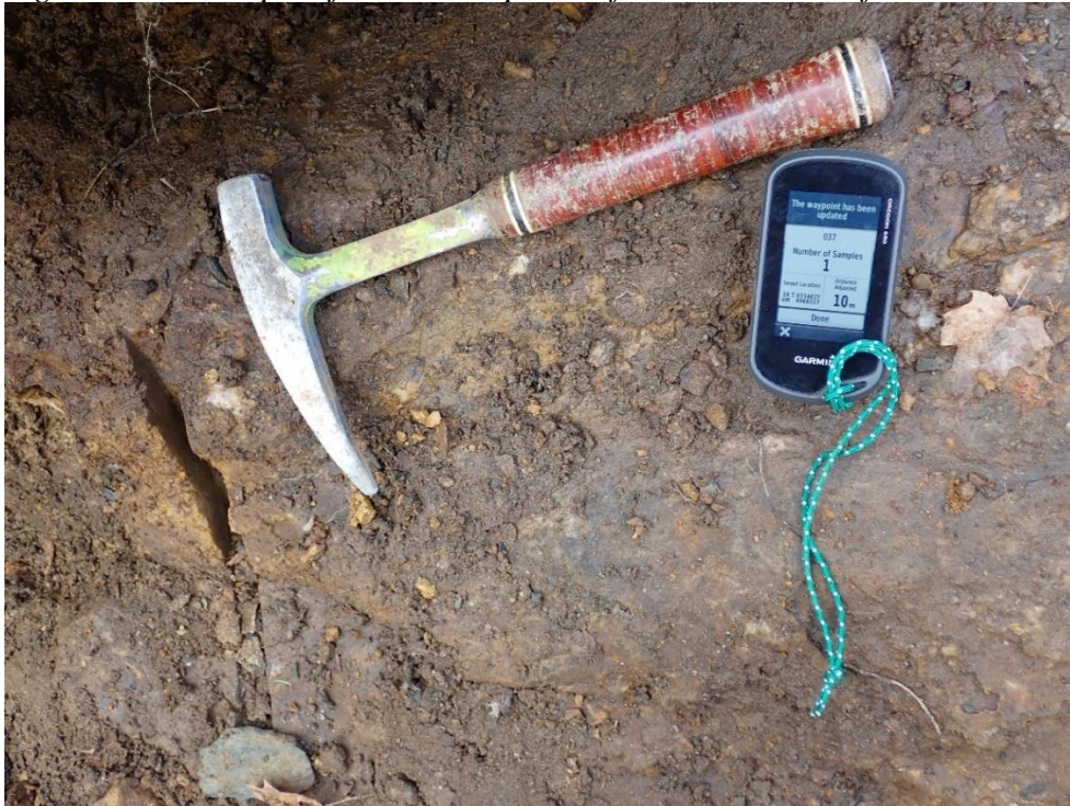
Figure 24: Outcrop 4 of Trench Map 2, High Grade Zone of gossanous Iron Formation with quartz veins, ferricrete, and limonite. Assay results from R.Waring on March 11, 2019 resulted in 67.6g/t Au (Sample 48423-LV4), 25.8g/t Au (Sample 48423-LV6), and 25.6g/t Au (Sample 48423-LV2), hammer for scale: 33cm
