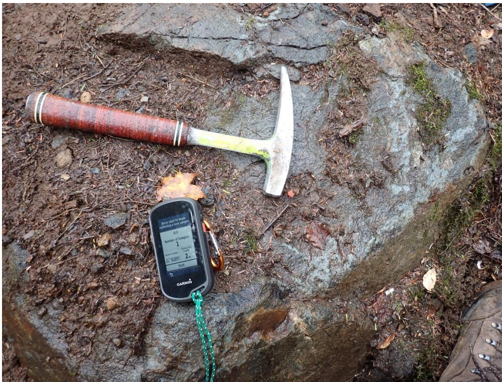
Figure 6: Outcrop 3 of Trench Map 1, Mafic Dike (Unit 3abc on MNDM Map Easton 2001), with foliation: 220/88° NW, hammer for scale: 33cm.
