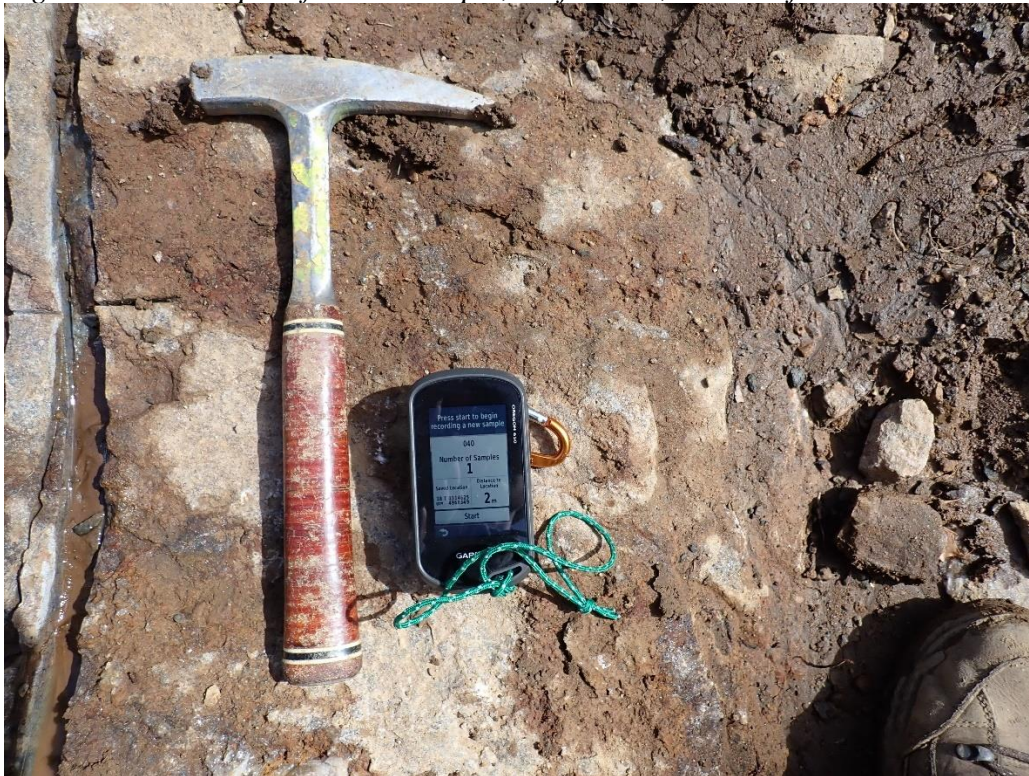
Figure 28: Outcrop 8 of Trench Map 2, Iron formation with quartz veins, hammer for scale: 33cm.
