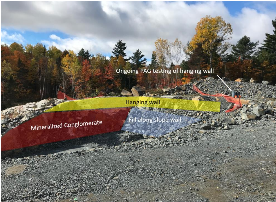
Figure 15. Trench 1 bulk sample section
