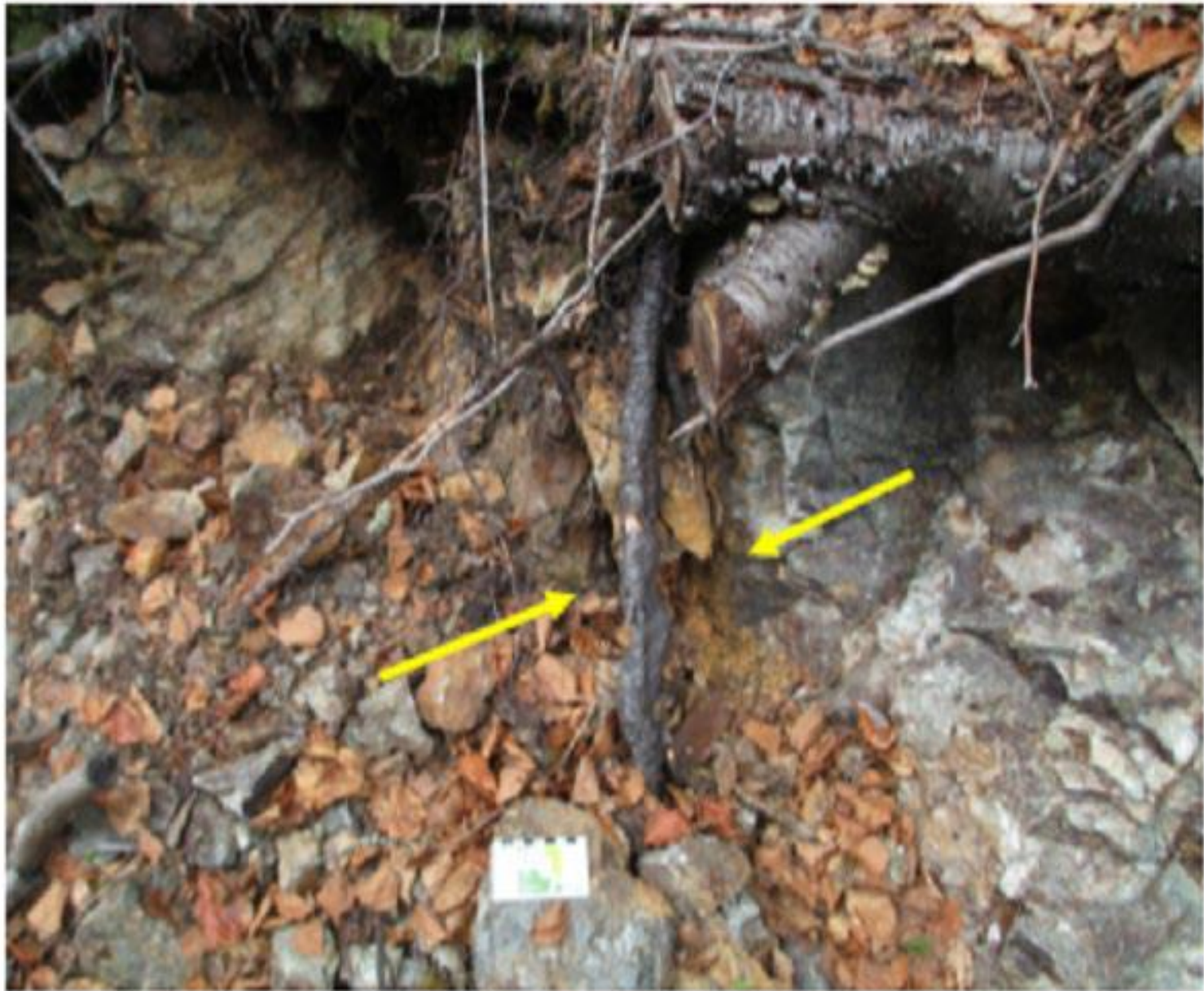
Quartz vein (between arrows) that strikes 264^{\circ} and dips 85^{\circ} (approximate UTM location: NAD83, Zone 17, 470158E 5344248N). Outcrop is east facing.
